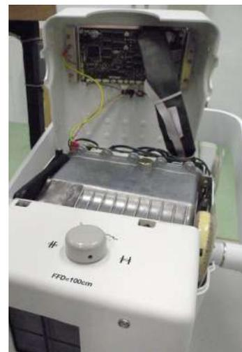
4. Open the Hinge Lock located at the top of the Detector Assembly in order to access to the X-Ray Unit connector plate and disconnect P1 and J1.
