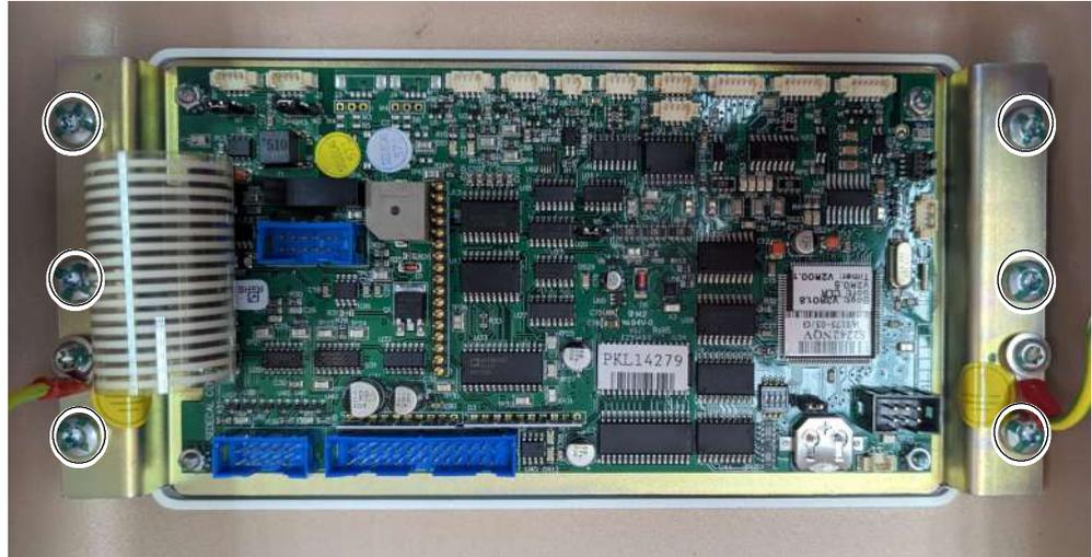
5. Re-install the plate support to the new Cover with the Hex screws.
