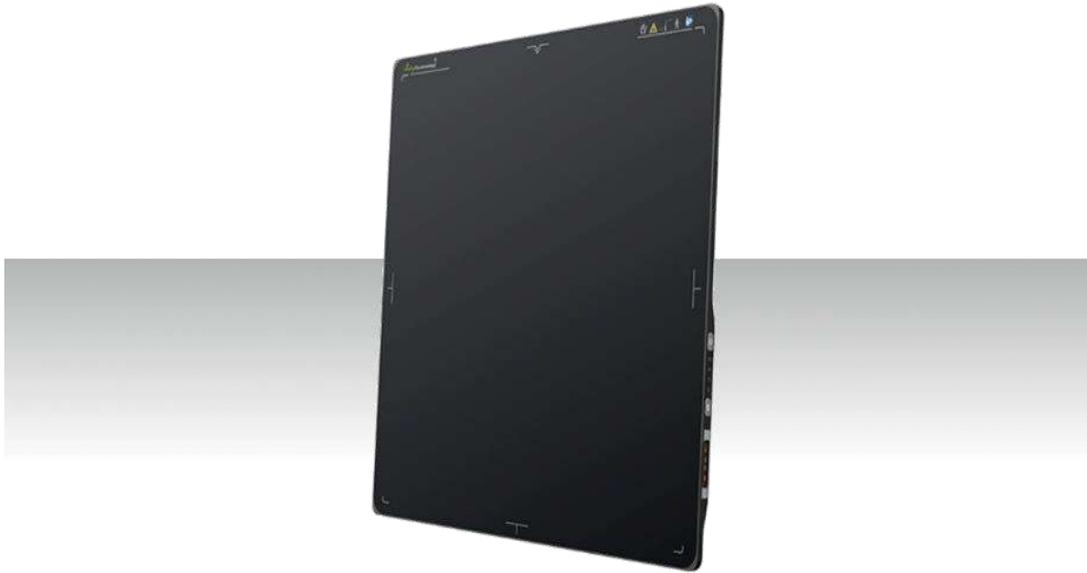
Designed to provide the highest quality of X-Ray images with an active matrix of 2,304×2,800 pixels and **100µm pitch** (CSI).
