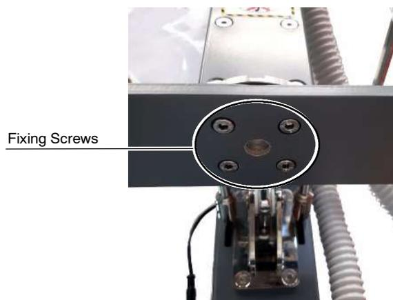
2. Verify that the eight (8) screws attaching rotation mechanism to the chassis are also in place and are properly tightened. There are four (4) screws on the front and four (4) screws on the back side. There is no specification for the torque on these screws as the load is transversal to the screw, but they have to be fully tightened.
