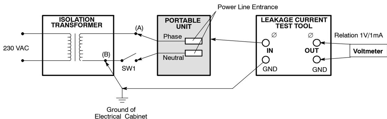
5. As shown in Illustration 7-1, the Voltmeter is set to  $V\sim$  and connected to the Test Tool at the **OUT** points. Connect **Ø (IN)** to a metallic part of the Portable Unit. Connect **GND (IN)** to the Ground of the Electrical Cabinet and to an output of the secondary of the Isolation Transformer (B).
