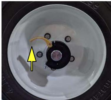
4. Take out the wheel of the shaft, replace it and install the lock ring again.
