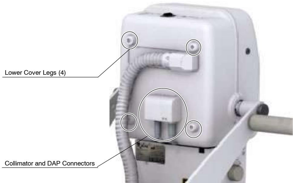
6. Carefully remove the Lower Cover. Pass the Power / Communication Harness through the Lower Cover window.
