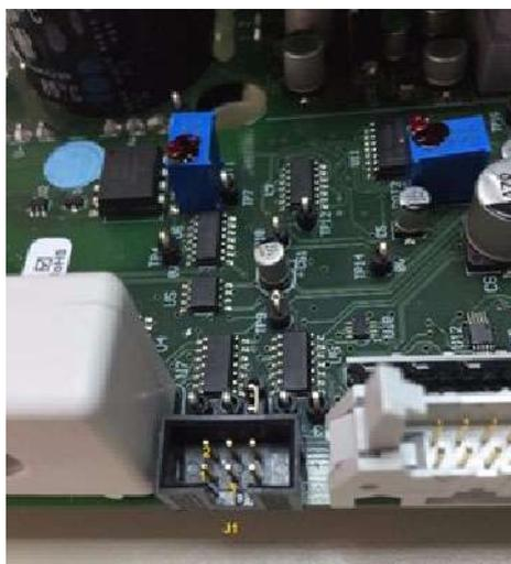
5. If the value of the resistance on the Control Driver are correct, disconnect the ribbon cable from J10 of HV Transformer and measure resistance on the following points of the HV Transformer:
