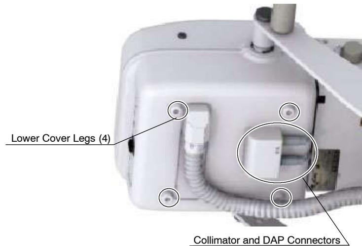
8. Carefully remove the Lower Cover. Pass the Power / Communication Harness through the Lower Cover window.
