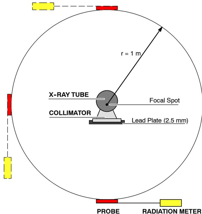
1. On the Portable Unit Console, select the following parameters: 125 kVp, 50 mAs (20 mA , 2.5 s).
