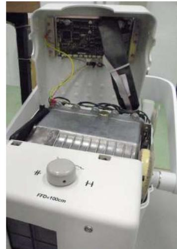
4. Unplug all the cables connected to the Portable Control Board (A3175-05).
