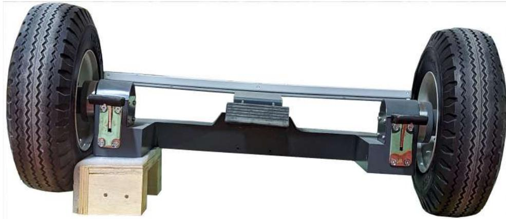
3. Open and remove the lock ring that holds the wheel.
