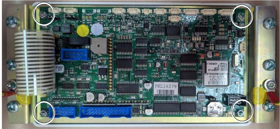
6. Remove the License by pushing and pulling it, and install it in the new Portable Control Board.
