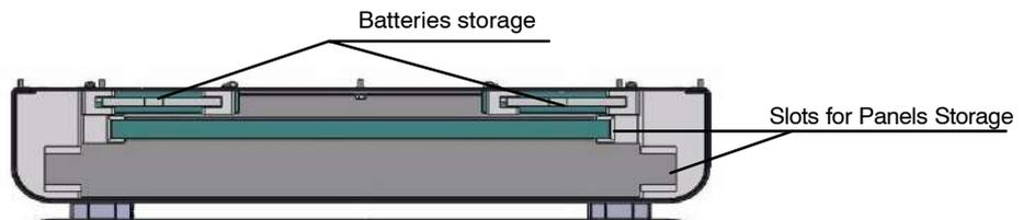
Detector Basket Hatch is available with an opening to allow the internal storage of the Detector Frame with Handle in case of large panels of 43 x 43 cm (17" x 17").
