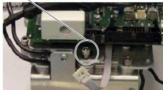
5. Disassemble the Shunt Plate and the Resistor.
