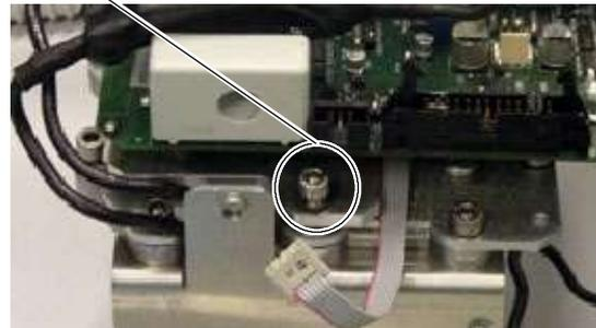
8. Pass the TA cable through the red (round) Current Transformer, crimp the round connector included in the kit. Pass the TB cable through the grey (square) Voltage Measurer. Attach cables with Tie Wraps when needed.
