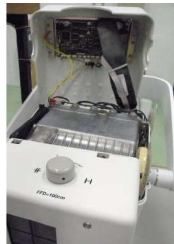
4. Disconnect the Collimator cable from the Lower Cover of the Unit and the DAP cable if connected.
