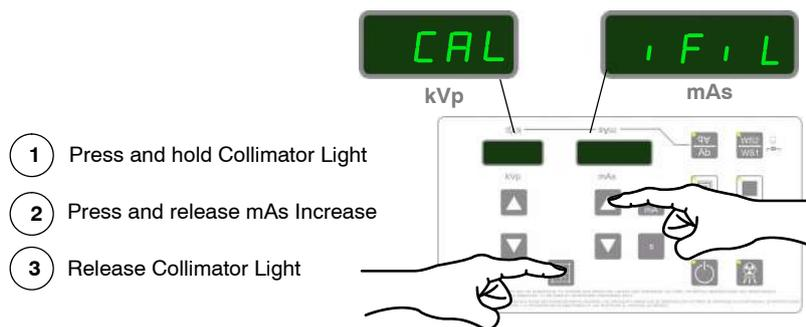
2. Select: 40 kVp, “Large Focal Spot” (led blinks), and 20 mA in Large Focal Spot (by pressing the mAs push-buttons). During Calibration the mAs Display shows the mA value.
