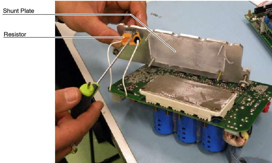
6. Remove old silicone on the Shunt Plate and apply a new layer on its surface. Assemble the new Control Driver Board (A3189-07) to the Shunt Plate by screwing the Resistor and the IGBT screws.
