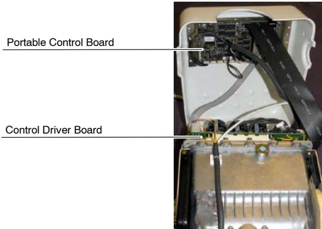
3. Connect Oscilloscope to the Portable Control Board (A3175-05) as indicated in *Section 3.1*.
