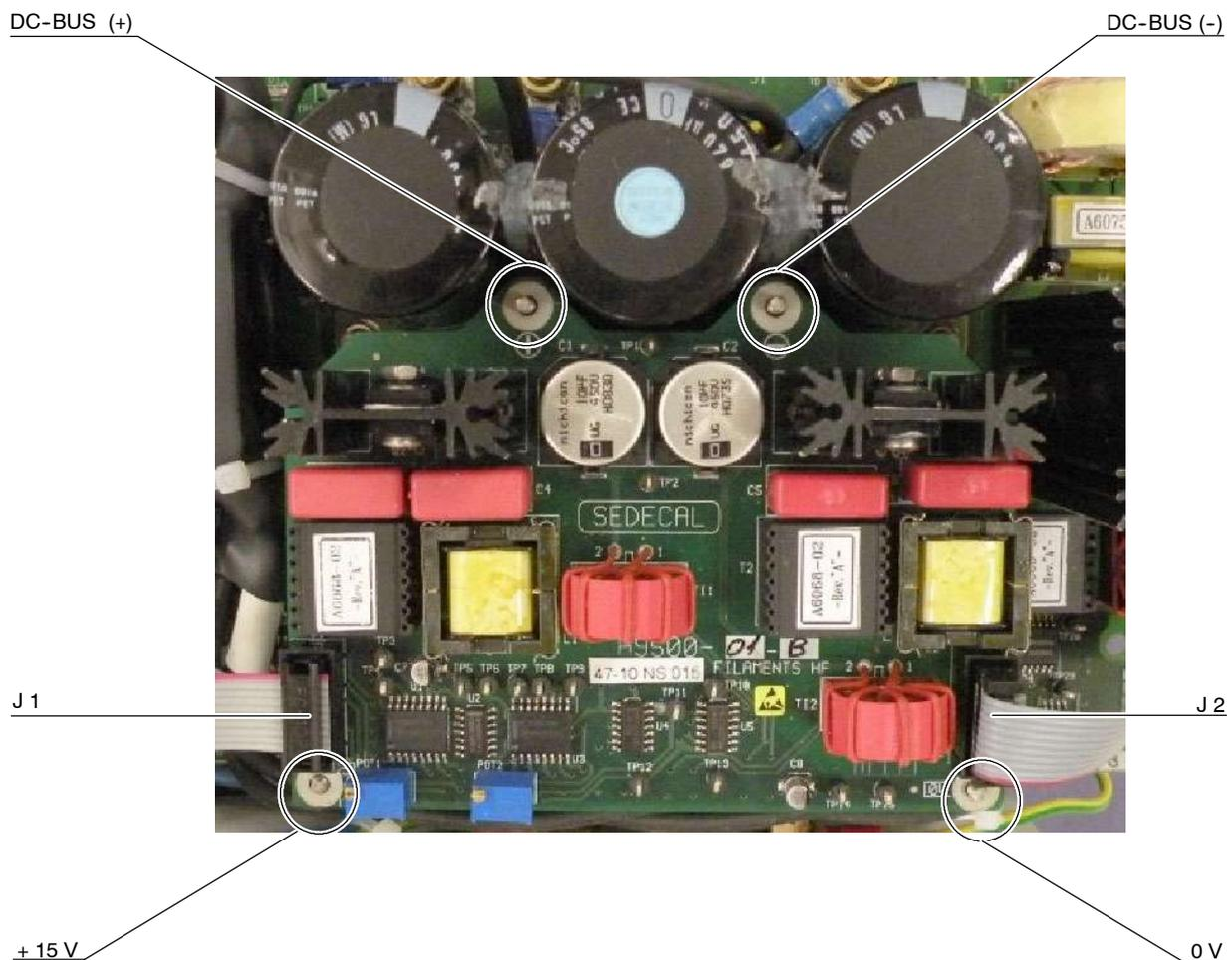
4. Replace the Filaments HF Board (A9500-01), reconnect and assemble in reverse order.
