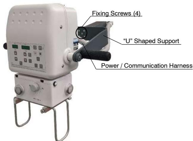
5. Remove the two (2) shaft assemblies from the “U” shaped support at both sides of the X-ray Power Unit.
