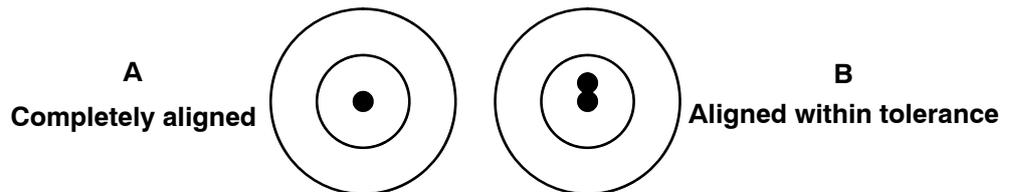
If the top ball is outside the first circle, correct the position of the X-Ray Unit. Repeat the process until the perpendicularity is correct.
