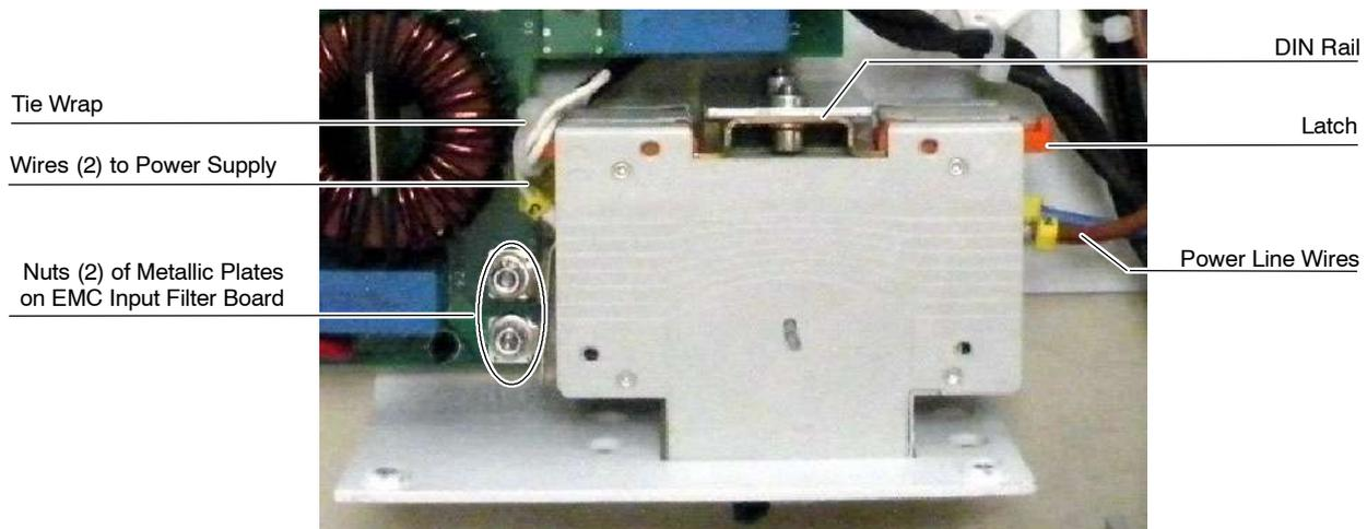
6. Replace the Circuit Breaker, reconnect in reverse order and assemble the X-ray Power Unit as described in *Section 6.3.16.1*.
