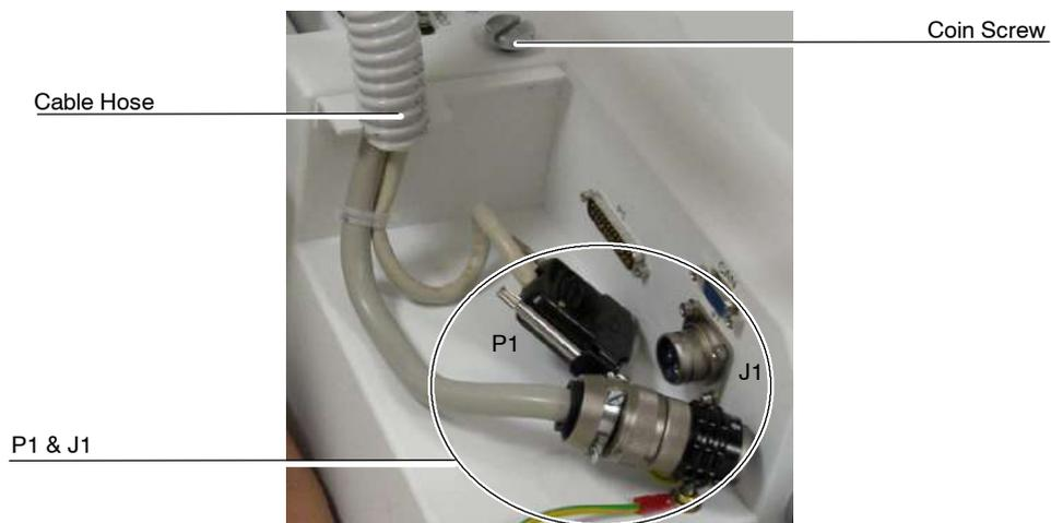
5. Release the Power / Communication Harness from the Cable Clamps attached to the Arm.
