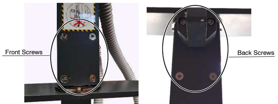
3. Check that the X-ray Power Unit is fixed to the “U” Shaped Support and that the Shaft Assembly is in place: Check that the Lock Nut is tightened enough for the X-ray Unit to stay still in a specific position, and enough for the X-Ray Unit to be easy to move, and that the Locking Washer Tooth is securing the Lock Nut.
