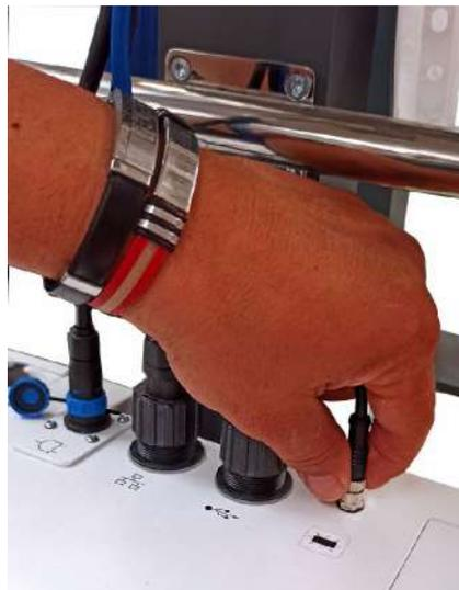
7. Carefully take out the LED Cable through the Cable Gland.
