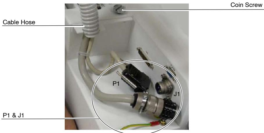
3. Carefully take out the Cable Hose from its entry.
