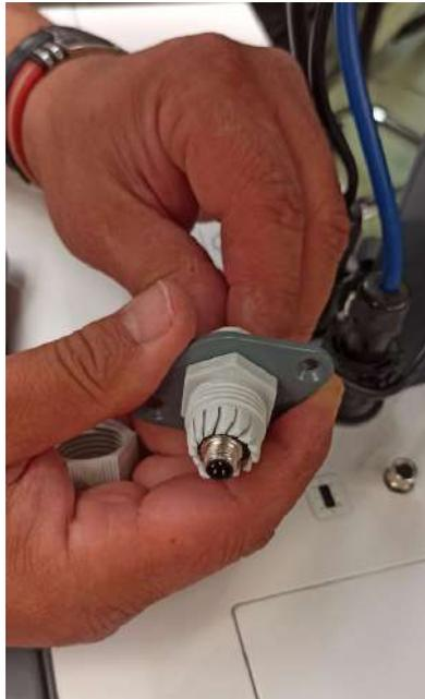
8. Pull up the LED Plate with the cable from the LED Plate window through the Chassis column.
