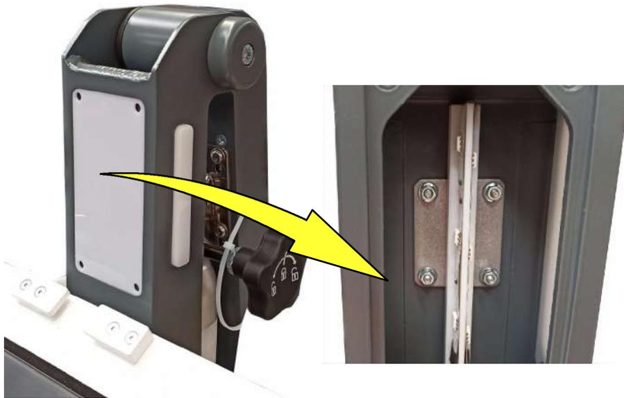
4. Remove the four (4) nuts that attach the LED Plate support to the chassis. Use a 3 mm socket wrench.
