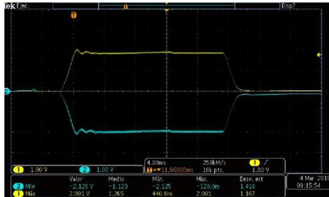
CH1: kV+ & CH2: kV- at 40kVp
