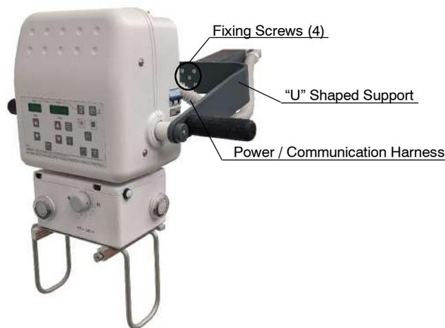
**2. Method-2 for disassembling the X-ray Power Unit from the Arm, only for equipment with optional “Quick Disconnect”.**
