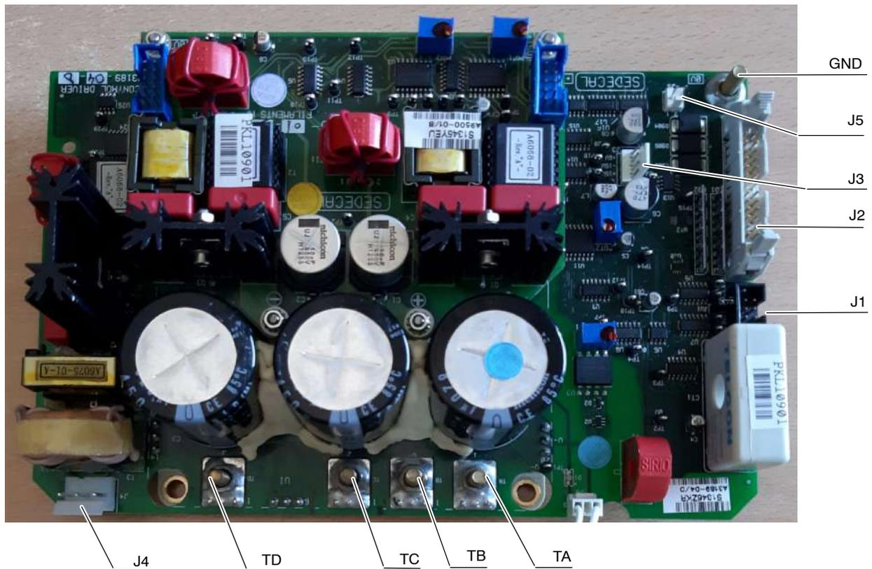
3. Cut the Tie Wraps when needed. Cut the round connector of the TA cable and take it out through the red (round) Current Transformer and take out TB cable (it is not necessary to cut this one) through the grey (square) Voltage Measurer.
