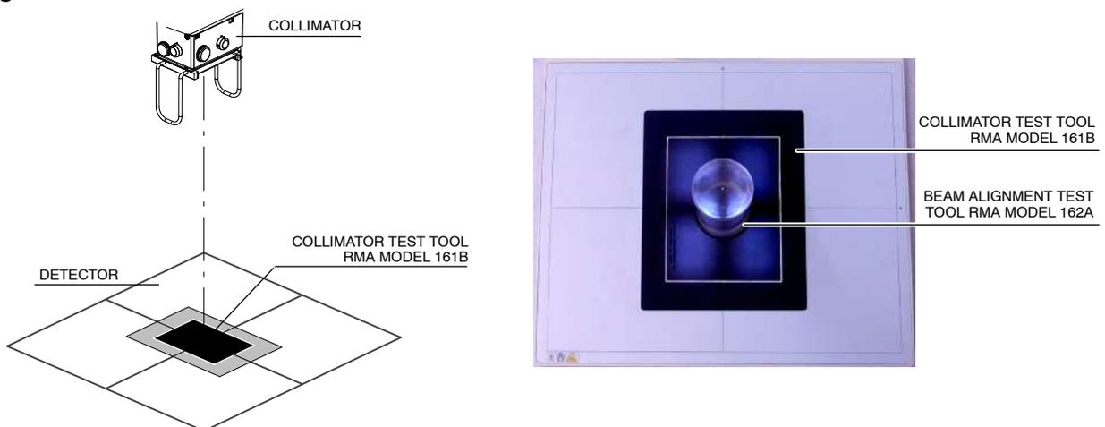
7. Make an exposure at 55 kVp / 5 mAs (10 mA / 0.5 s) and Small Focal Spot.
