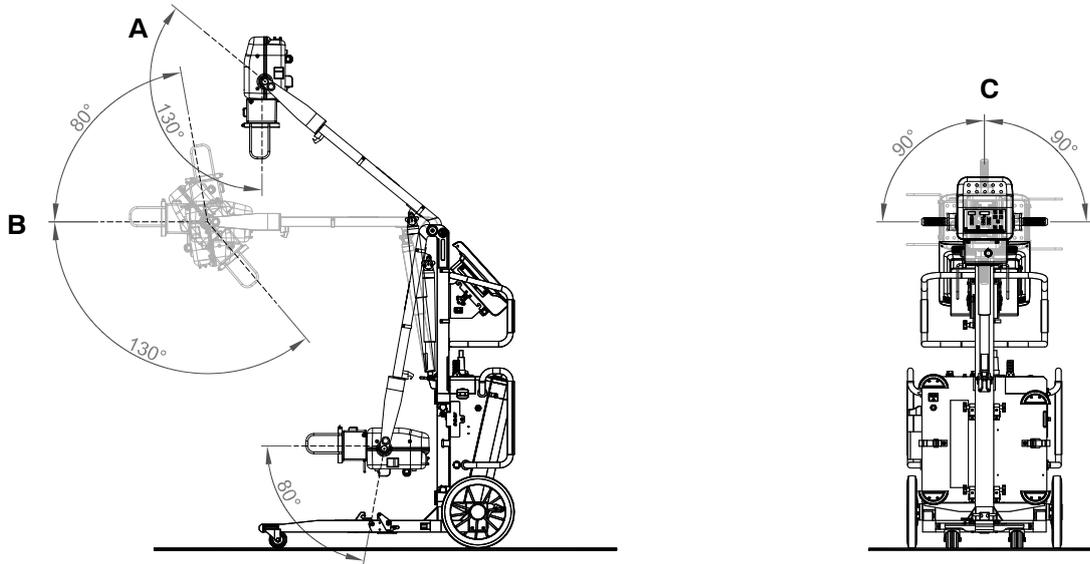
A. Rotation of the X-Ray Unit with reference to its Support
