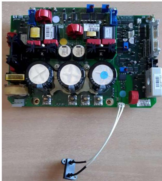
7. Secure the Control Driver Board assembly to the HV Transformer with the two screws removed before.
