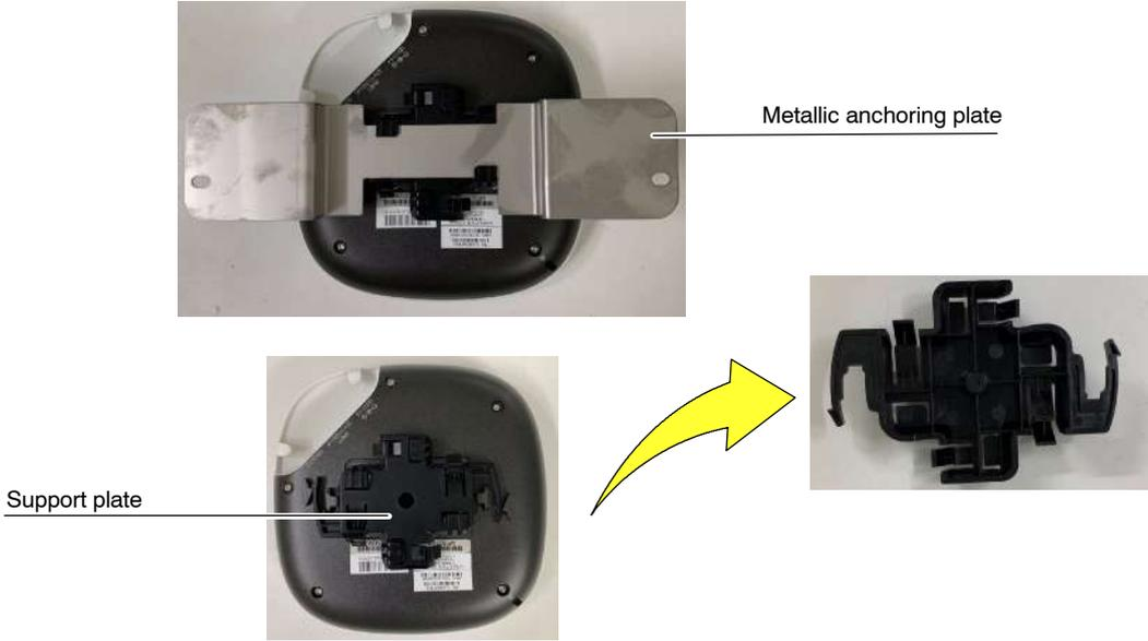
8. Replace the Access Point following the previous step in reverse order. Plug the LAN Cable connector into the socket labelled as “ENET 57V, 350mA” and the DC Supply Cable Connector into the socket labelled as “12V, 1A” (refer to the next pictures).
