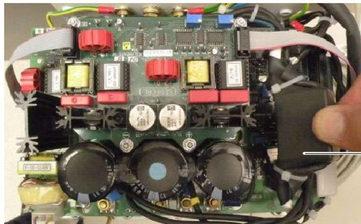
4. Pass the cable through the new large Heat Shrink and then through one of the new small Heat Shrinks.
