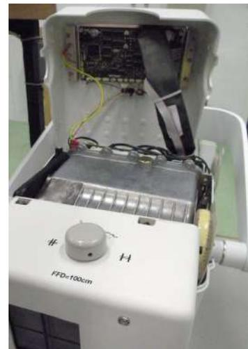
3. Cut the tie wrap of the inner part of the Cover. It is not necessary to disconnect any cable from the Portable Control Board (A3175-05) for Upper Cover replacement.
