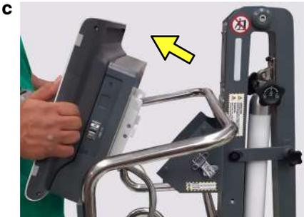
3. Dismount the Detector Basket. Unscrew the four (4) lock knobs located at both sides of the column that attach the Column of the Trolley to the Detector Basket.
