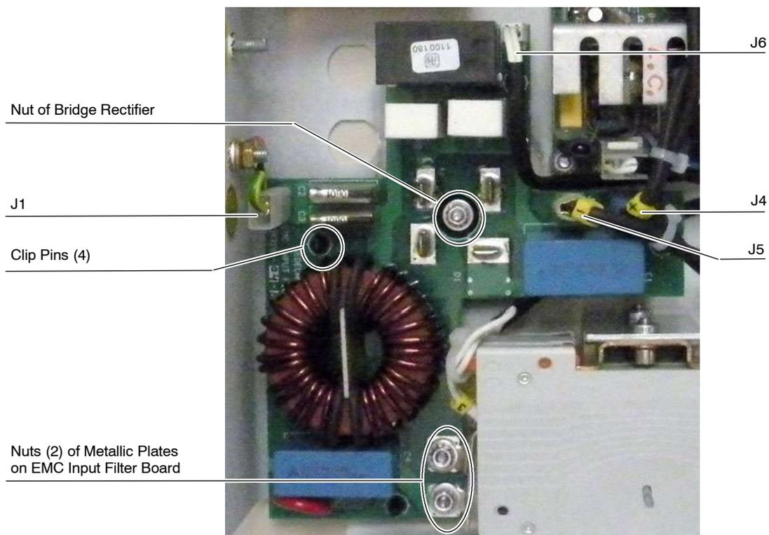
7. Remove the two (2) metallic Plates from the old Board and install them on the new Board.
