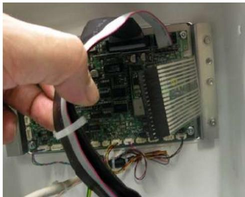
5. Unscrew the nuts located at each corner of the Portable Control Board and remove it.
