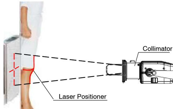
The Laser Positioner can be activated by pressing the “*Collimator Light*” push-button. It remains lighting for 30 seconds before it switches off automatically (lighting time can be configured from 10 to 50 seconds during installation by the Service Engineer).
