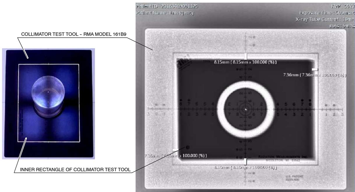
If any edge of the X-ray Field does not coincide with the edge of the inner rectangle means a misalignment of the Light Field with respect to the X-ray Field. The maximum misalignment allowed is 2% of SID (for SID 100 cm = 2 cm tolerance) for both axes.
