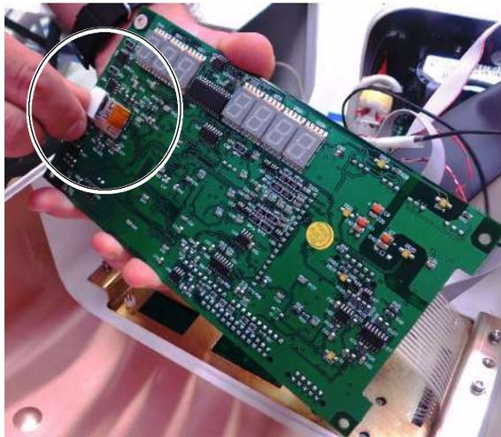
7. Install the new Portable Control Board.
