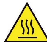
CAUTION HOT SURFACE
