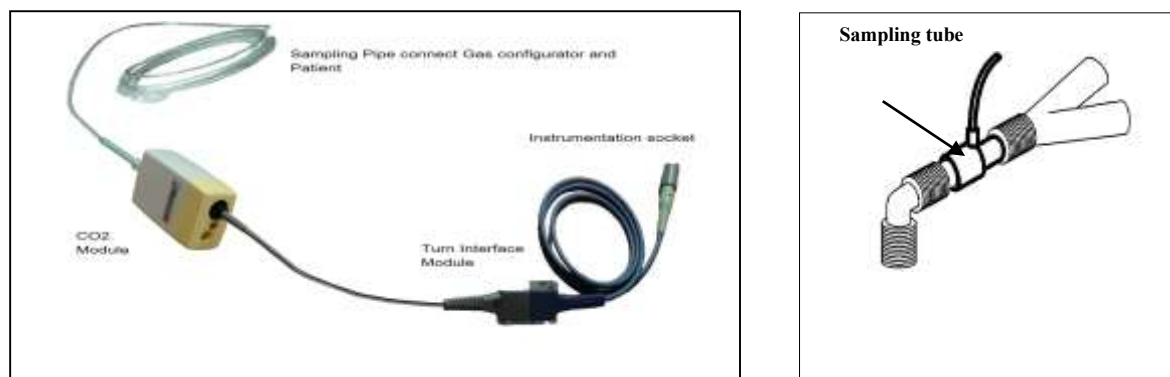
Figure 23-4ISA™ Sidestream Analyzer (ISA CO 2 ) CO 2 Connection Schematic
