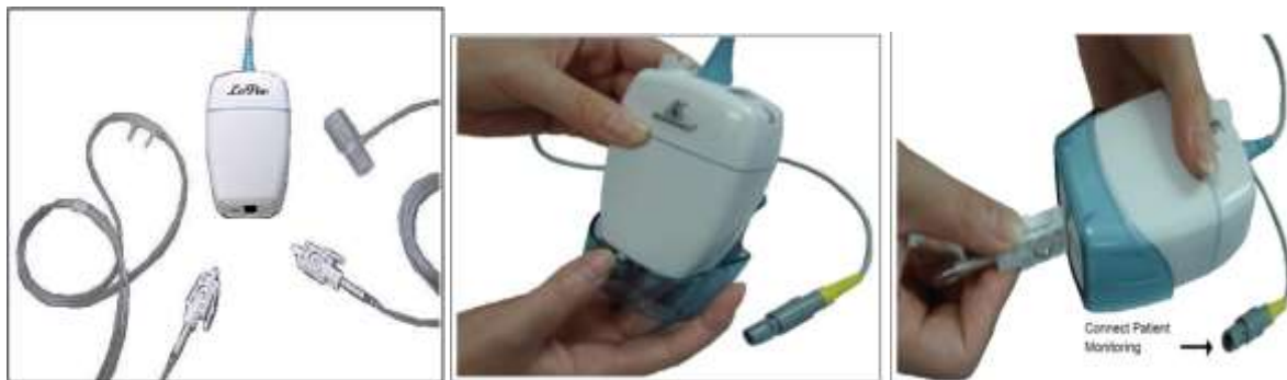
Figure 23-3 Sidestream CO2 module connection schematic
