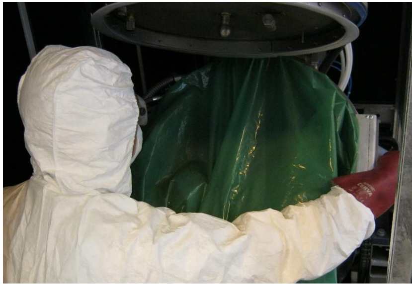
Fig. 53 – Checking Waste Bag Ring's Position
