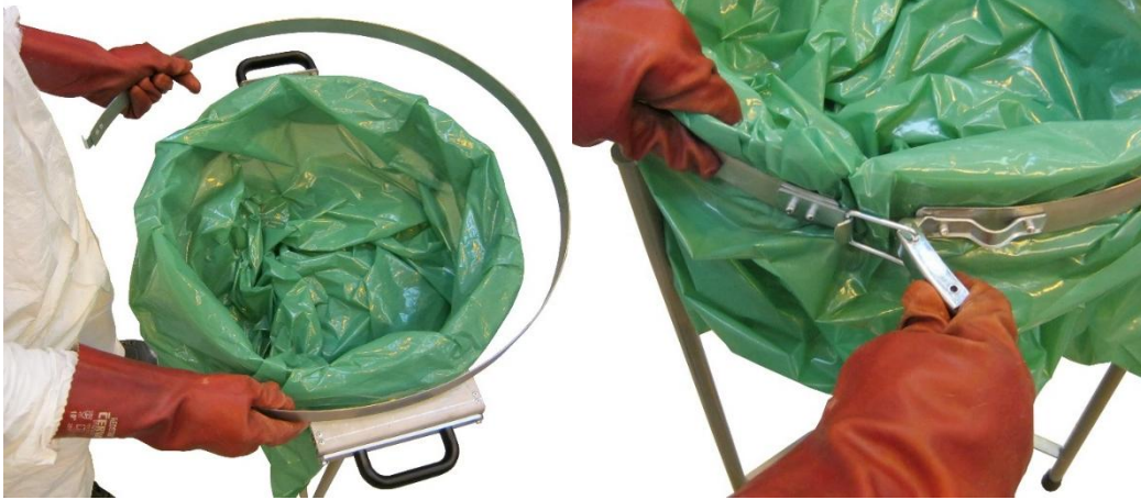
Fig. 66 – Placing and Closing Waste Bag Ring's Rim Lock
