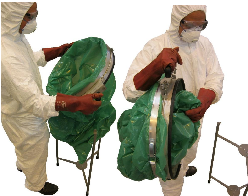
Fig. 67 – Preparing Waste Bag Ring for waste discharge
