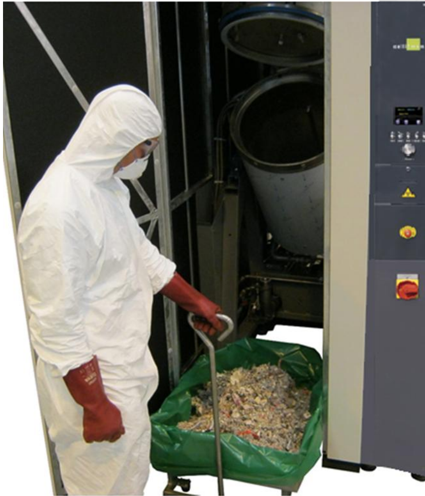
Fig. 51 - Removing Trolley from Loading Area
