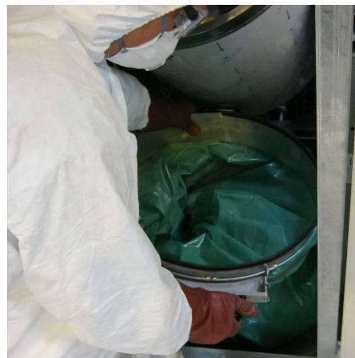
Fig. 58 - Removing Waste Bag Ring from Chamber's Flange
