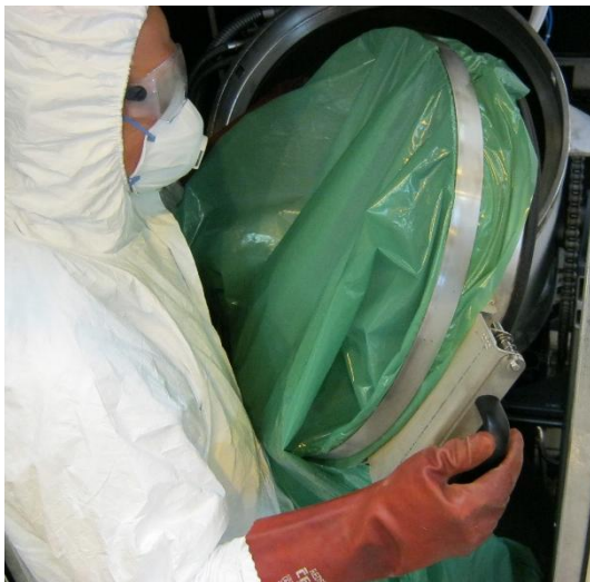
Fig. 58 - Removing Waste Bag Ring from Chamber's Flange
