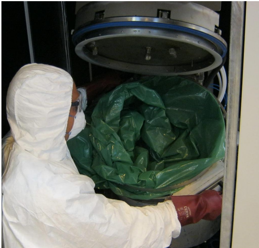
Fig. 52 – Placing Waste Bag Ring on the Chamber
