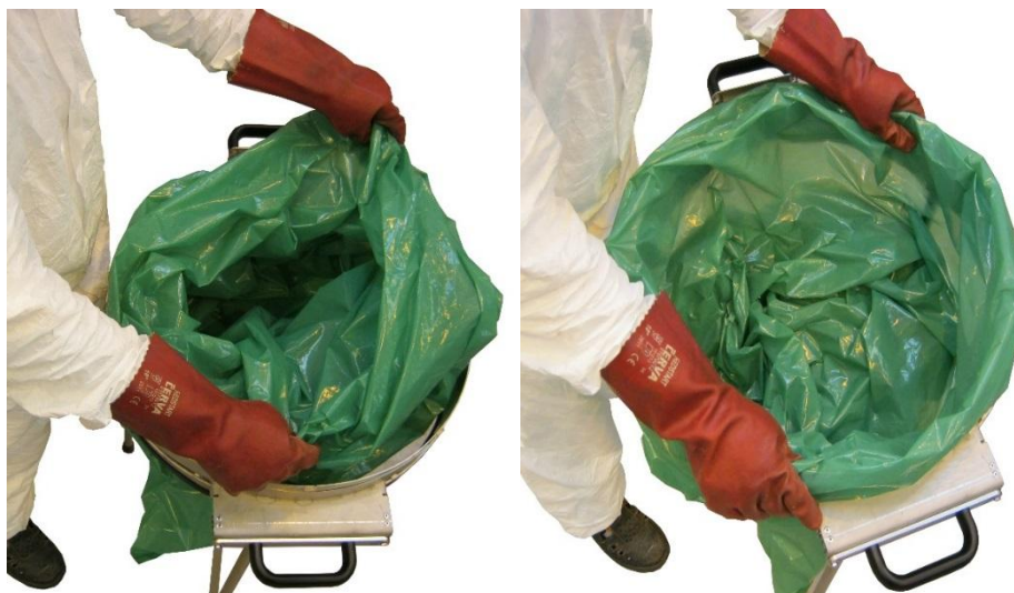
Fig. 65 – Pacing waste bag onto Waste Bag Ring
