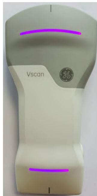
Figure 3-20. LED steady magenta light
