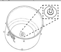
The white pivot pin disk (PTFE material) is located inside the bottom of the cuvette.
