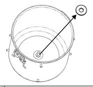
▶ Pull out the pivot pin disk by hand.
