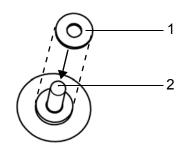
it onto the pivot pin (2). Push it fully downwards to the bottom.
