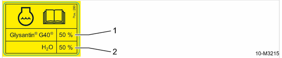
Fig. 30 Recommended mixture ratio for coolant
