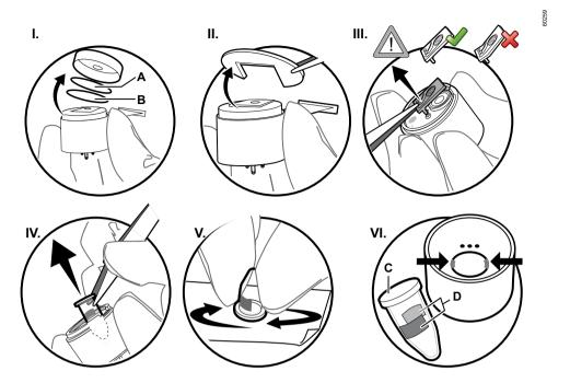
During calibration of the PID, the gas detector identifies when there is dirt on the lamp and displays a corresponding warning. If this warning is displayed, the lamp window must be cleaned. Silicone-free disposable nitrile gloves and the DrägerSensor PID cleaning set (order no. 83 19 111) must be used for this. The cleaning set is for single use.
