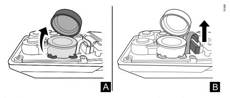
b. Carefully pull out the sensor and only then detach the flexstrip from the printed circuit board.
