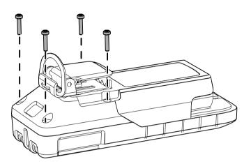
i Dräger recommends first tightening the two lower housing screws and then the two upper ones.
