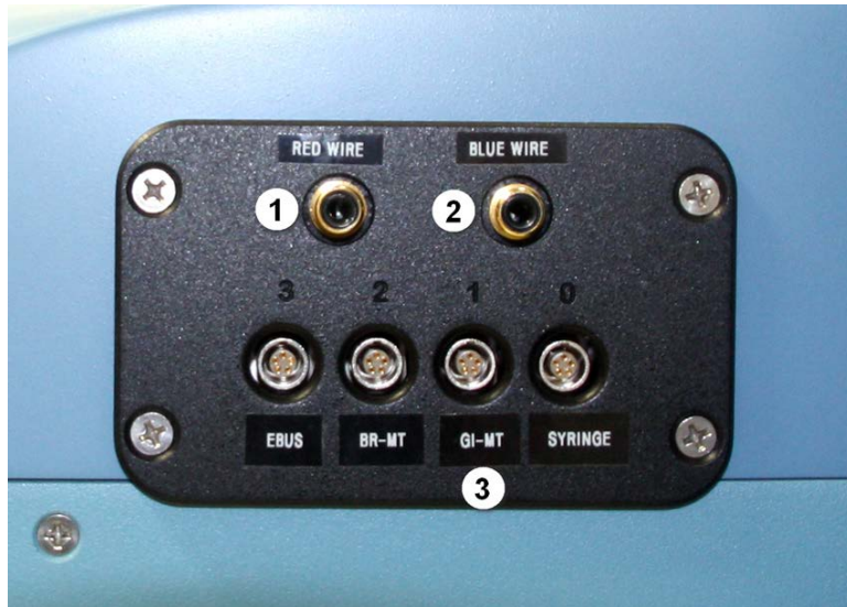
Figure 3-9: Tool connection outlets
