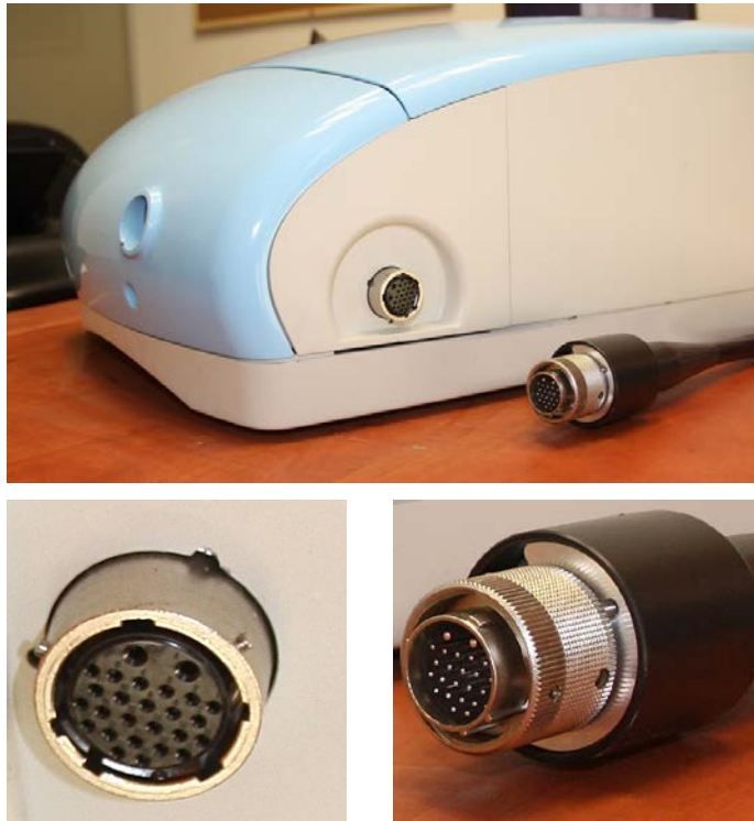
Figure 4-6: System side and scope side connectors
