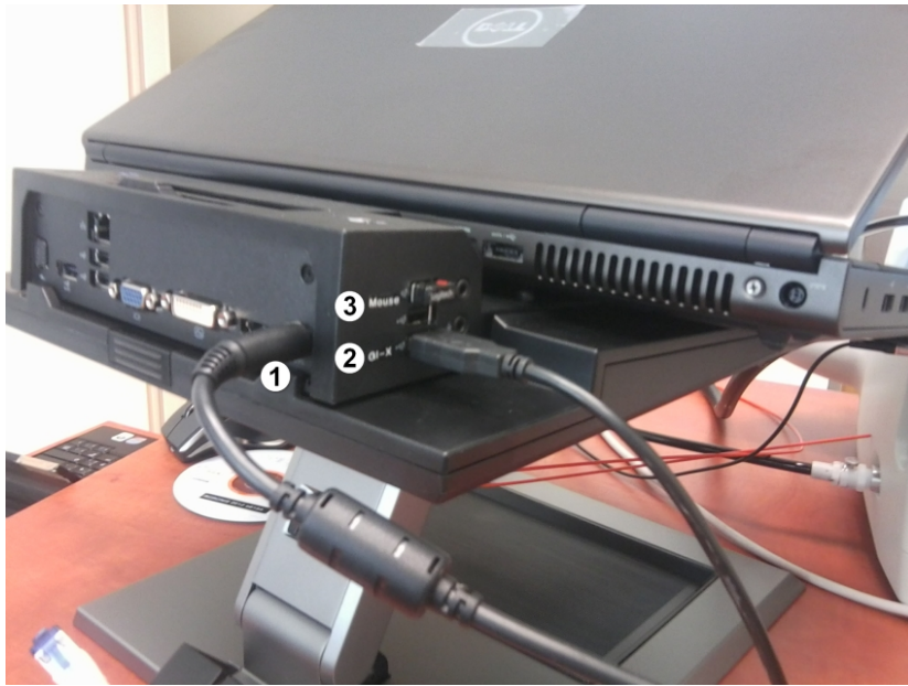
Figure 4-4: Docking station connectors
