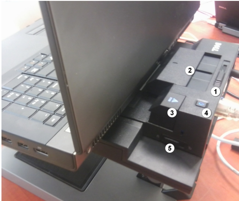
Figure 4-3: Attaching and securing laptop to docking station
