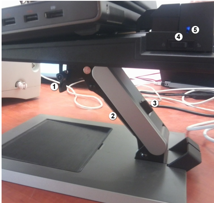
Figure 4-5: Adjusting the docking station
