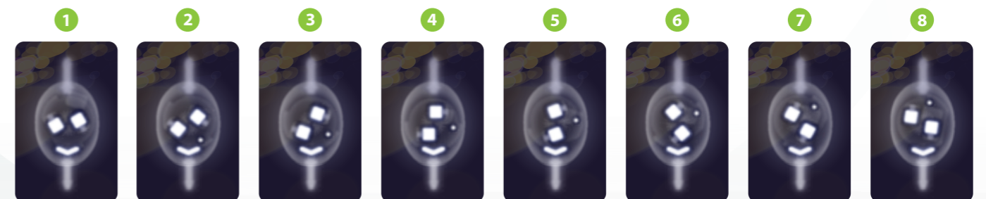
X-ray image of Sphera Pro for the 08 pressure settings, showing the inlet and outlet connectors, both magnets, the direction arrow, and the indicative mark for the valve laterality.
