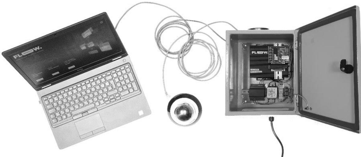
TrafficEmbedded is able to perform in a number of different topologies and setups (as described in the following sections), however, in this phase we will limit ourselves to the simplest configuration - we will connect the computer directly to the internal network of the TrafficEmbedded unit.
