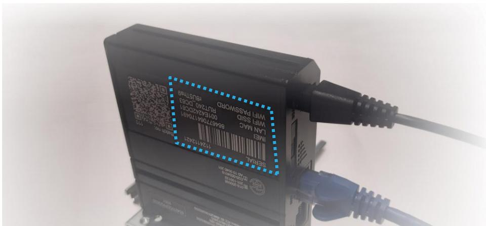
Alternatively, you can connect your computer to TrafficXRoads via LAN cable. Access the LTE modem web interface at **192.168.1.1**
