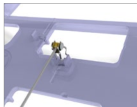
Figure 3c: Removing Coupler and FMT from the holding frame
