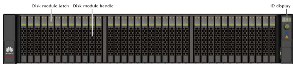
Figure 3-25 Front view of a 2 U 36-slot smart NVMe disk enclosure
