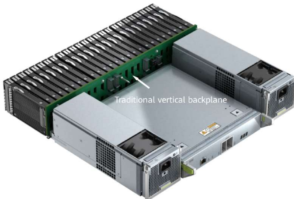
Figure 3-27 Traditional vertical backplane
