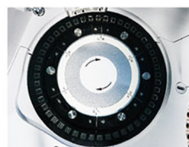
Reaction Tray 37±0.2°C, real-time monitor.
