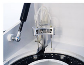
Washing Probe Independent 3-step washing system.
