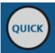
By pressing and holding the QUICK key, you perform the quick spin. The centrifuge will run as long as you hold the key pressed. Time of run is displayed on the time display. When you release the key, the braking procedure of the rotor is activated and the centrifuge stops.
