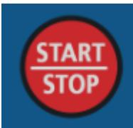
By pressing the START/STOP key, you start or stop the run of the centrifuge. After the expiration of set running time or after manual stopping of the centrifuge by pressing the START/STOP key again, the braking procedure of the rotor is activated and the centrifuge stops. The next run is possible, when the rotor stops completely.
