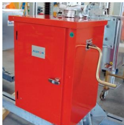
Painted mechanism for added protection against corrosion
