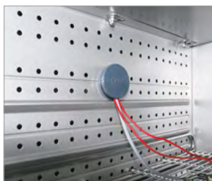
Access port with silicone plug
