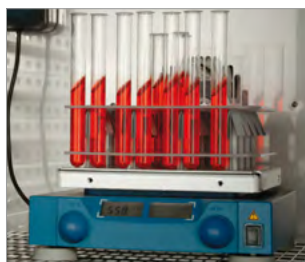
Shaker operation in the chamber
