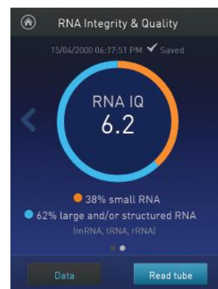
Figure 6. A proprietary algorithm is used to report a quality score representative of the ratio of small and large and/or structured RNA in the sample.
