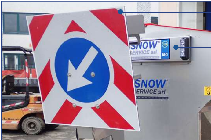
Steel license plate support with pair of strobe lights
