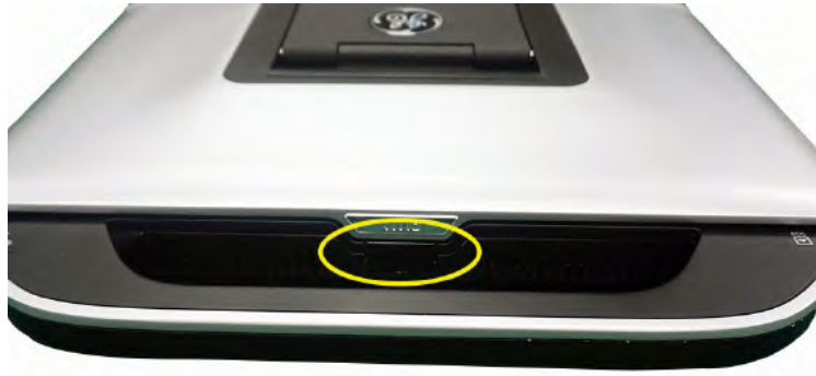
Figure 3-7. Unlock the LCD
