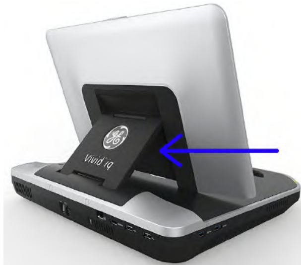
Figure 3-8. The pinch point
