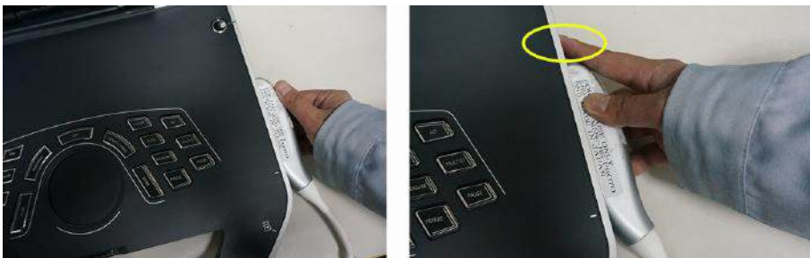
Figure 12-2. Probe connection to Vivid iq
