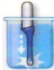
Figure 12-15. Probe suspended in disinfectant basin
