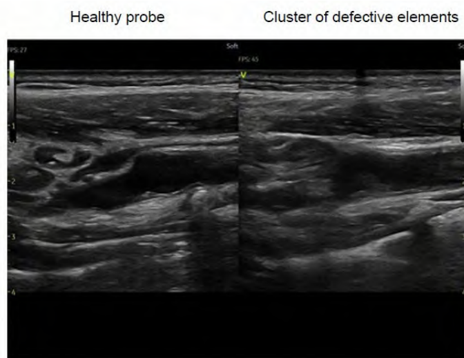
Figure 12-28. Example of image degradation for a linear probe
