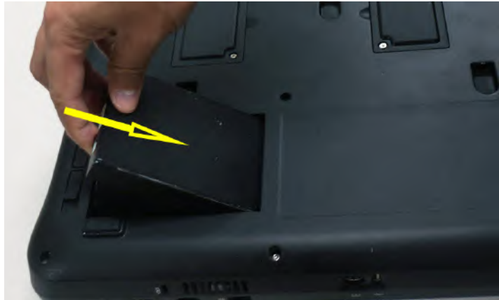
Figure 3-31. Place the battery in the battery box
