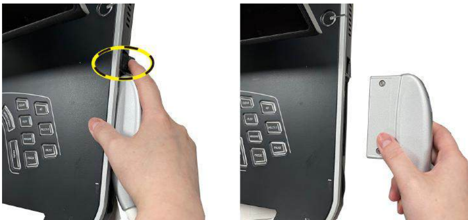
Figure 12-4. Probe disconnection from Vivid iq
