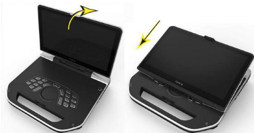
Figure 3-10. LCD adjustment up/down
