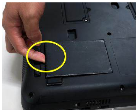
Figure 3-30. Remove the battery
