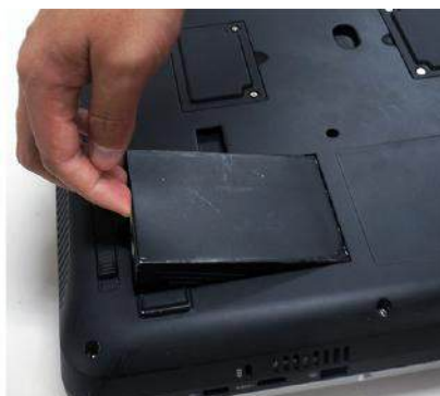
Figure 3-30. Remove the battery
