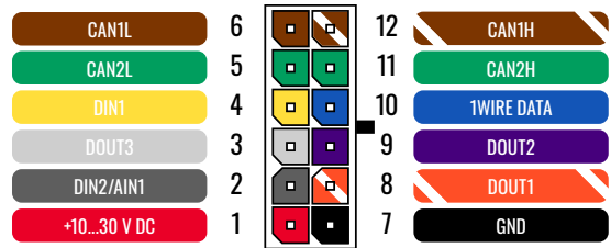
FMB150-QKIB0 pinout
