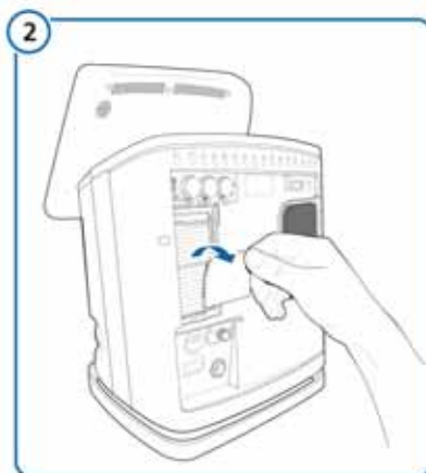
Remove and replace air intake dust filters
