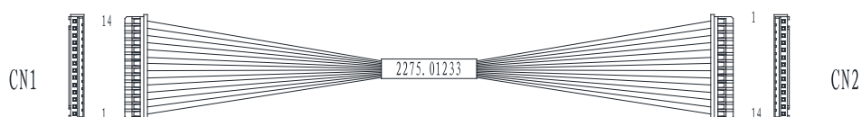
Figure 5-13 Key Panel to Knob Board Cable
