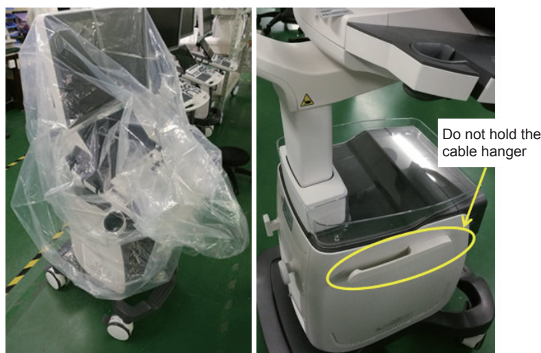
Figure 2-8 Pulling Out the System
