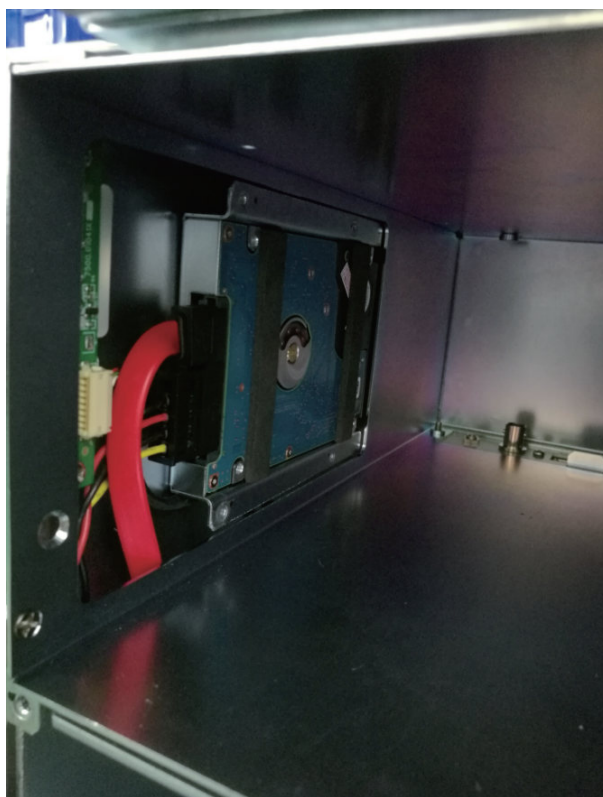
Figure 4-18 Removing Hard Disk
