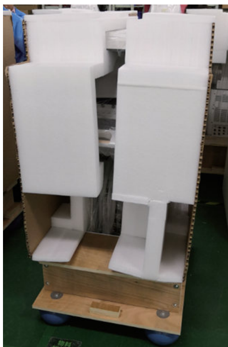
Figure 2-5 Removing Cotton Protectors
