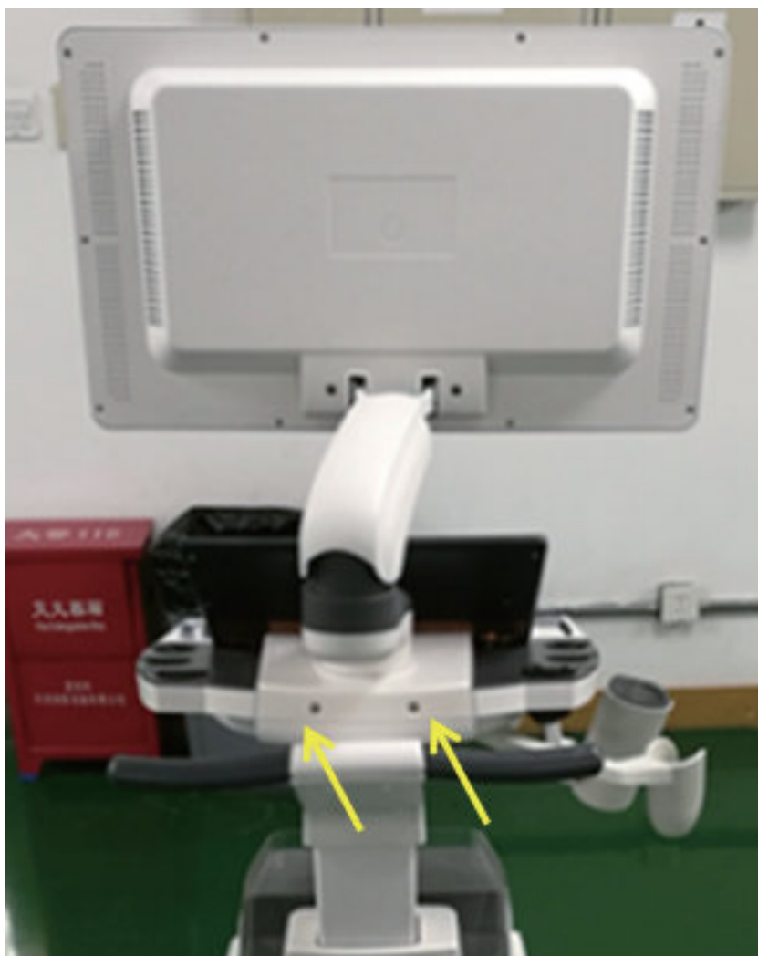
Figure 4-4 Removing Display Arm
