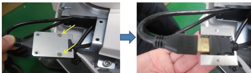
Figure 4-6 Removing Arm Assembly
