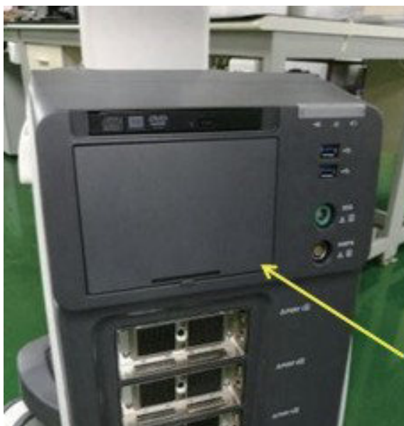
Figure 4-16 Removing the Cover of the Printer Compartment
