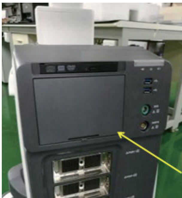
Figure 4-19 Removing the Cover of the Printer compartment
