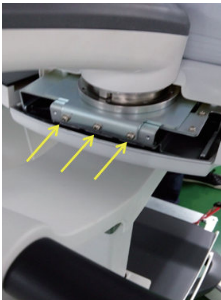
Figure 4-7 Removing Arm Fixed Screws
