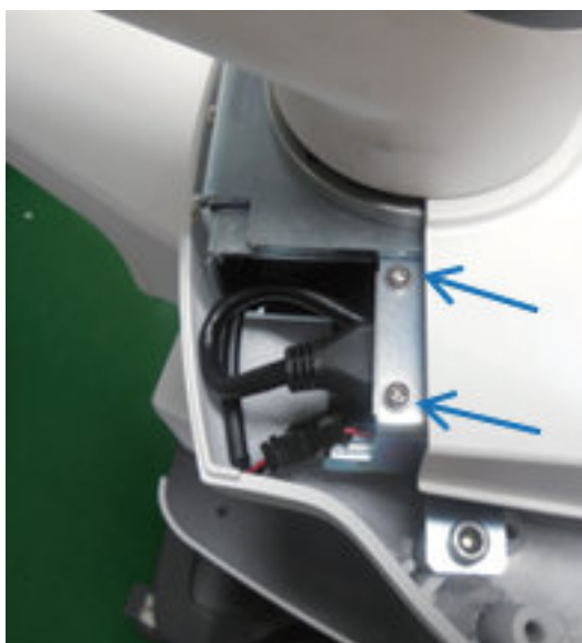
Figure 4-5 Removing Cable Fixing Plate
