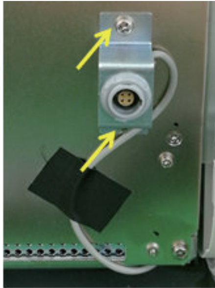
Figure 4-24 Removing Footswitch Socket
