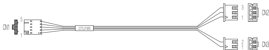
Figure 5-49 Internal IO Board to Main Board PS-ON & Starting Switch Cable
