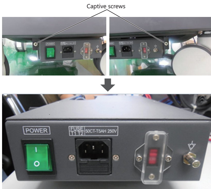
Figure 4-35 Removing the Isolation Transformer
