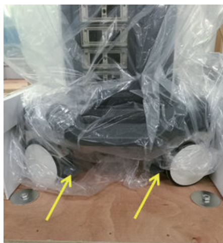
Figure 2-7 Releasing the Four Casters
