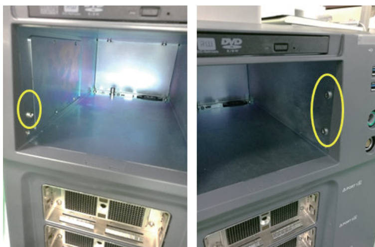
Figure 4-20 Removing Screws Fixed Printer Front Panel
