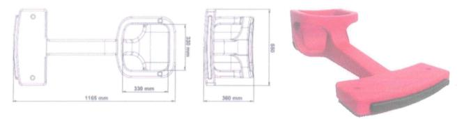
The swing seat is made of LLDPE material, suitable for 1 child. The maximum user weight is 55 kg. Dimensions: 420x485x325 cm.
