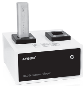
M10-103 Charger unit for 2 battery (without battery) • Mains voltage 100-240 Volts, 50-60 Hz, 0.9 A • Charging current 1.5 A • Charging voltage 9.6 Volts • Protections: Short circuit / Overload / Over voltage • 200 x 200 x 120 mm / 2500 g
