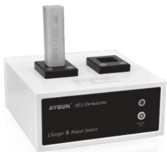
M10-105 Power supply and Charger unit for 2 battery (without battery) • Mains voltage 100-240 Volts, 50-60 Hz, 1.5 A • Charging current 1.5 A • Charging voltage 9.6 Volts • Power supply 12 Volts, 5 A • Protections: Short circuit / Overload / Over voltage • 230 x 230 x 120 mm / 3200 g
