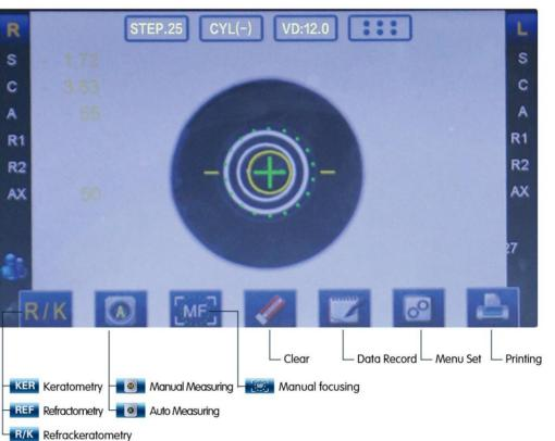
Intuitive icons provide the user an easier operating circumstances, and make the measurement become more convenient and the data to be measured more accurate and fast
