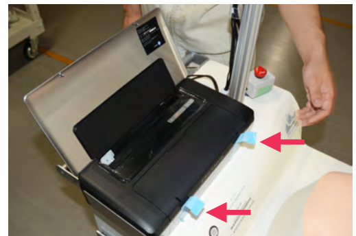
3, Peel off the tapes before using. *Ensure to turn on the printer AFTER turning on the main power of the simulator
