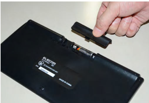
1, Set the dry batteries to case on the back of the keyboard. *At the time of delivery, sample batteries are enclosed.
