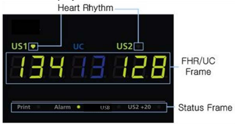
Fig. 5.2 Main Monitoring Screen
