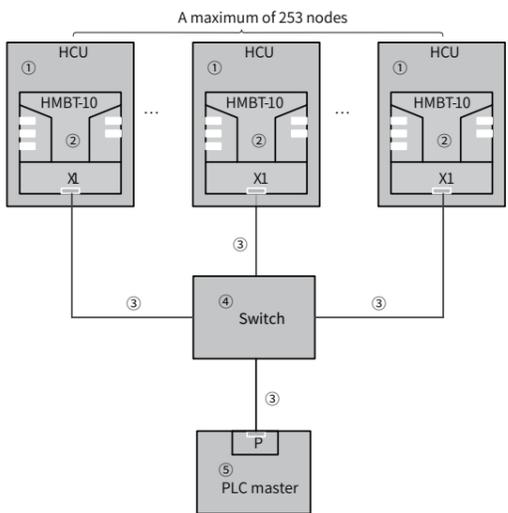
Figure5 Diagram of electrical connection for multiple modules
