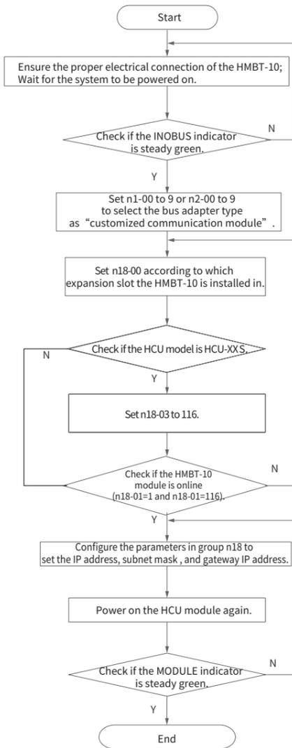
Figure6 Flowchart of HMBT-10 module configuration
