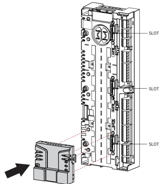
Step 2: Press the snap-fit joint ① of the HMBT-10 module inward into the slot, and fasten the grounding screw ② of the module with a Phillips screwdriver.
