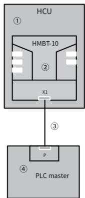
Figure4 Diagram of electrical connection for one module
