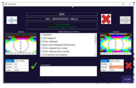
From version 1.2.12 Azimuth and Elevation out of limits are not flagged as errors. The field will be highlighted in amber to indicate a potential problem but the beam and light will be shown as good with a green tick. Candela and Colour discrepancies will still cause the beam and light to be failed.
