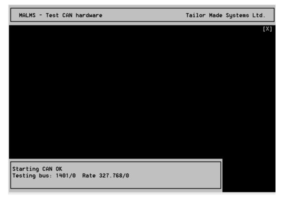
A failure is indicated below. Check the turntable is turned on. Check the cable is connected to the PC and the turntable. See also document *I-1112-A WST Troubleshoot CAN network problems.pdf*.
