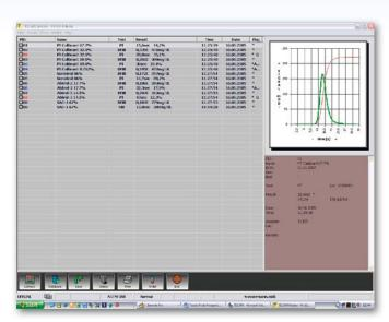
Receive results from instrument including the reaction curve which will help to validate before saving them into the database.
