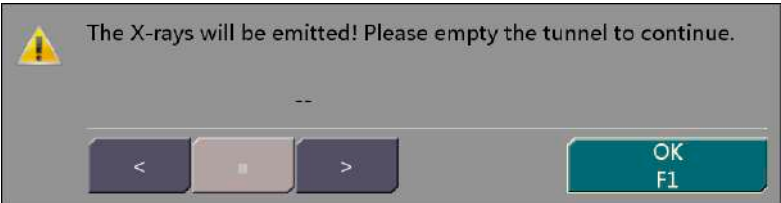
Figure 5-1 Prompt for Emptying the Tunnel
