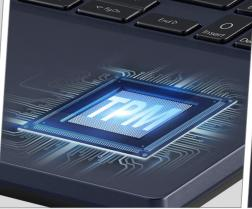
A dTPM chip securely stores authentication information used by software, such as password and importation transactions.
