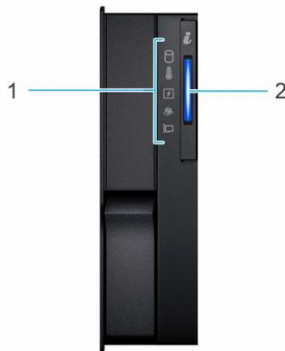
**Figure 8. Left control panel**
