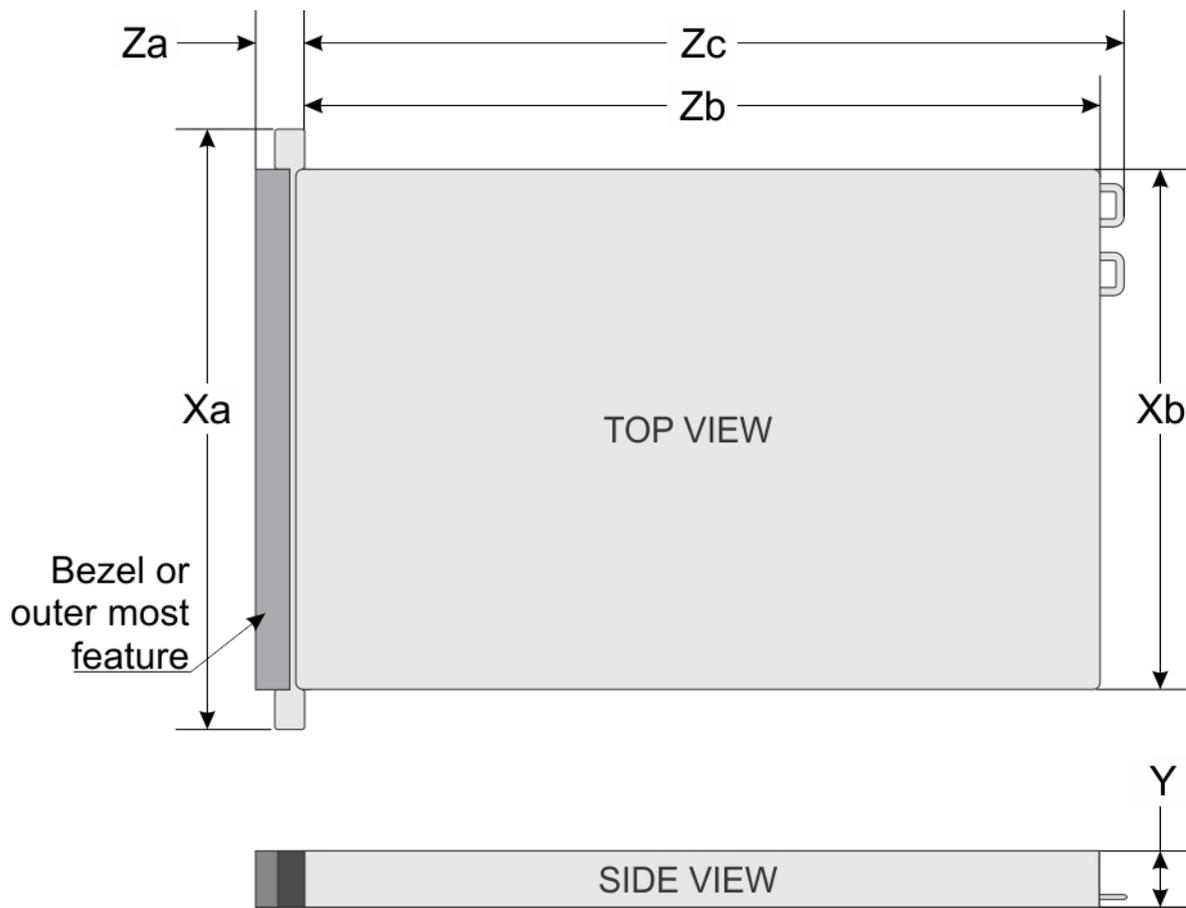
Figure 22. Chassis dimensions
