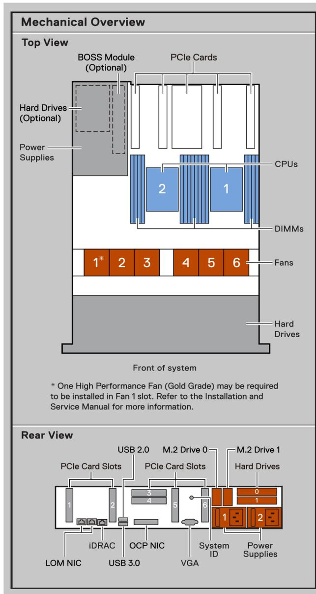
Figure 16. Mechanical Overview, Rear view
