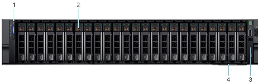
Figure 1. Front view of 16 x 2.5-inch SAS/SATA + 8 x 2.5-inch NVMe drive system
