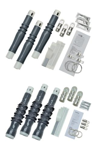
TE's Raychem Cold Shrink Terminations CSTI/O are made from a high performance, liquid silicone material which is specially formulated for excellent tracking and split resistance. The extra-long silicone stress cone is integrated within the termination which ensures correct positioning. Moisture sealing at the lug is integrated into the termination body, eliminating the need for additional sealing tapes.
