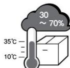
Where the temperature changes frequently (Normal temperature for operation of the machine is at the range of 10°C ~ 35°C, and the humidity is at the range of 30%~70%.
