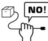
Always pull the power cord holding the plug and not the cord.
