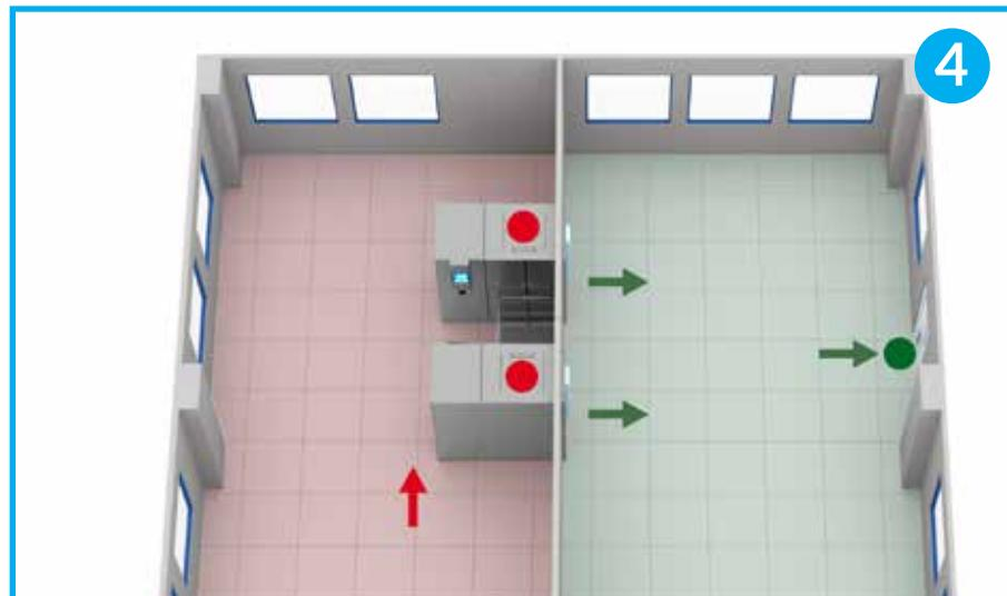
The mobile waste collection container is routed inside of the pre-chamber thanks to the **guided** movement of the device.
