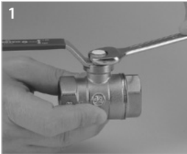
Remove the nut with the proper wrench
