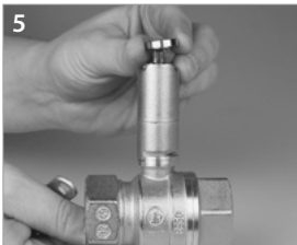
Insert the brass washer (included in the package)
