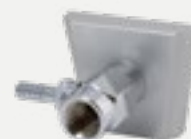
Anodized aluminum wedge for OHMEDA rail clamp bracket, with nipple threaded ISO G. 1/4" F. and hose connector Ø 6 mm (for medical gases) or Ø 7.5 mm (for vacuum).
