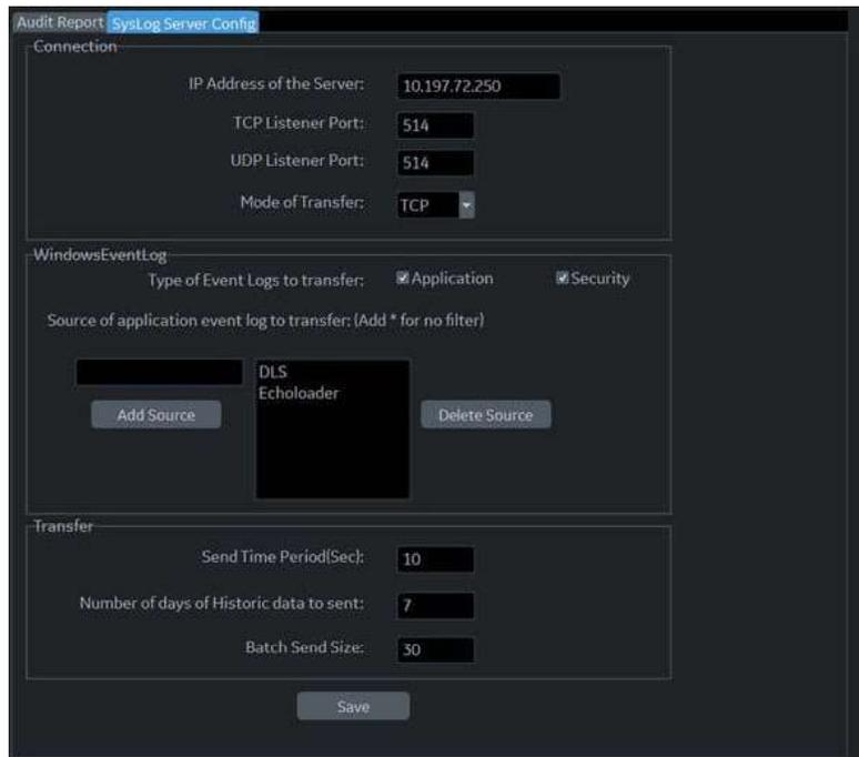
Figure 10-79. System Log Server Configuration
