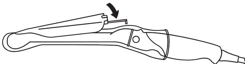
Figure 11-25. Disposable Biopsy Guide 5 degree Angle
