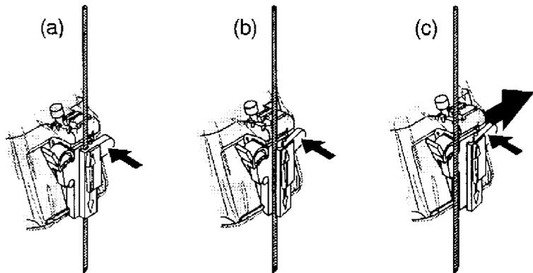
Figure 11-19. Release the needle from assembly
