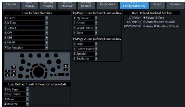
Figure 13-9. Set UGAP as any User-defined Hard Key
