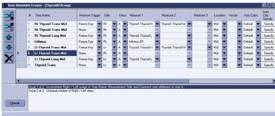
Figure 13-144. Rule Check Button and Rule Check Results
