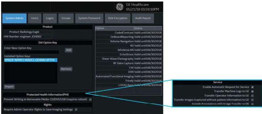
Figure 10-65. Remote Connectivity Deactivated; Service Fields Removed
