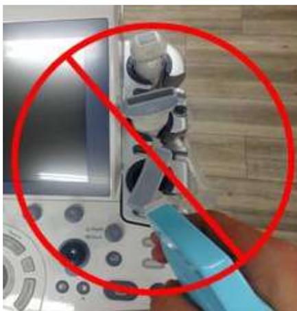
Figure 12-7. DO NOT Spray a Probe While in its Holder
