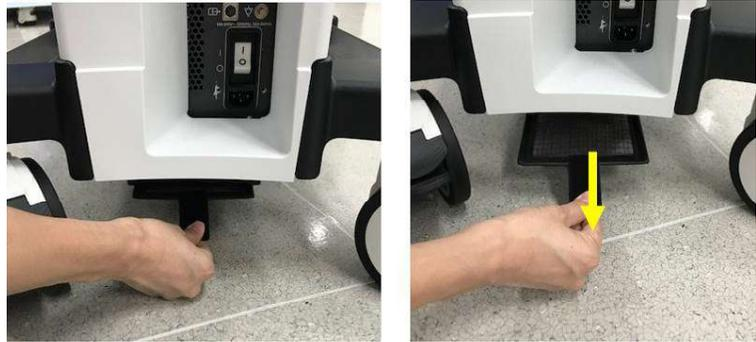
Figure 12-6. Air filter location
