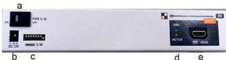
Figure 13-273. Input side configuration
