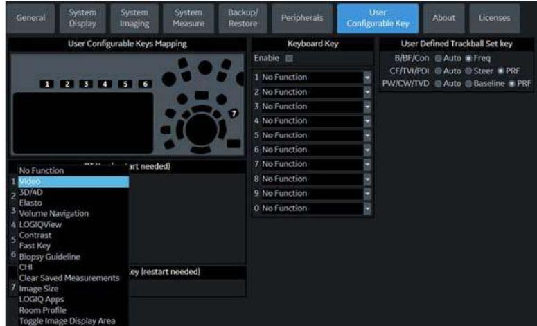
Figure 13-286. Assign LOGIQ Apps to a BT Key
