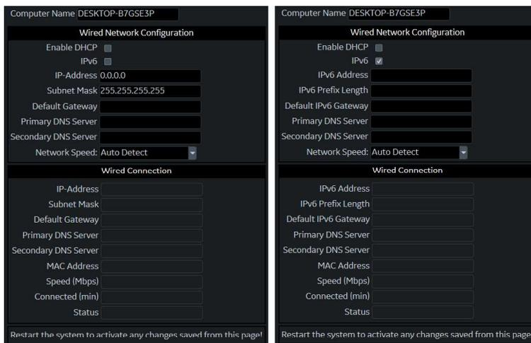
Figure 10-46. IPv4 and IPv6 Static IP Connectivity Menu
