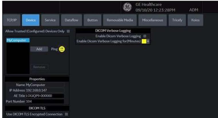
Figure 10-47. Connectivity Device Preset Menu
