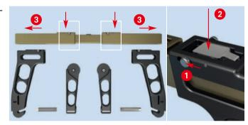
After disassembly, clean the rails, arms and threaded tubes manually, e.g. by using a brush. The springs in the upper arm at button should be cleaned too. If necessary, broken or damaged parts should be exchanged.
