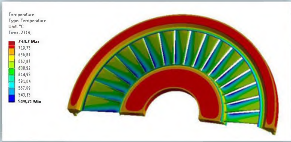
Distribution of temperature fields in the rotor diaphragm during heat treatment
