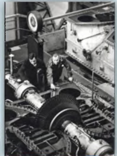
1985. The workers of Steam Turbine Aerodynamics Laboratory are preparing the model of ETND-2 turbine for testing
