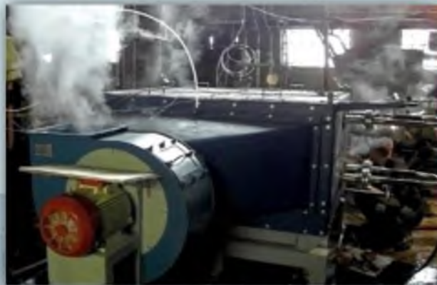
Recirculation cooling plant RCP-6.3 EMK.0155.000.00.000 for the third unit of the Rostov Nuclear Power Plant (emergency mode emulation)
