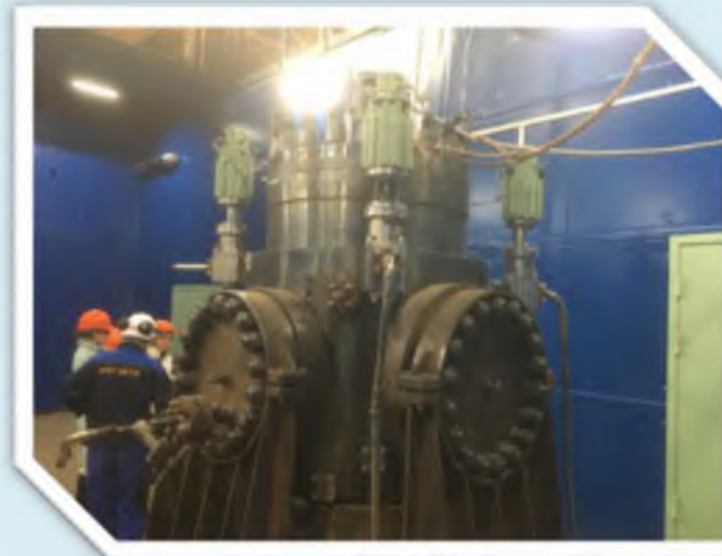
On of the testing spots of the Complex Test Rig KS10606 BZOK-600 and IPU PG are put on the test rig.
