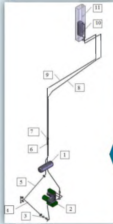
Large-scale model SPOT PG of the reactor unit LAES-2. Coolant heat capacity and power scale (1:110) 1 – steam generator/separator 2 – circulation pump 3, 7 – throttling flow meters 4, 5 – electric heaters 6 – main steam isolation valve 8 – steam pipeline 9 – condensate pipeline 10 – emergency cooling heat exchanger 11 – emergency heat removal tank
