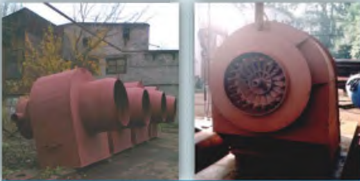
Oil-gas burner GMU-m with tubular gas distribution
