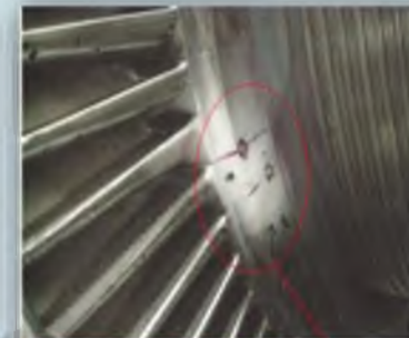
Crack in the blade root at the 4th stage of HP rotor of K-500-65/3000 turbine
