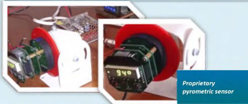
Layout of sensor installation for measuring the shaft train twisting value
