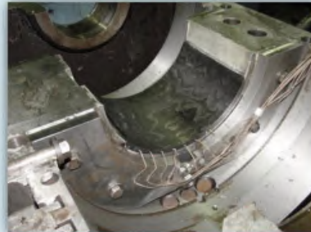
Installation of a journal bearing with the face made of new synthetic material on the test rig
