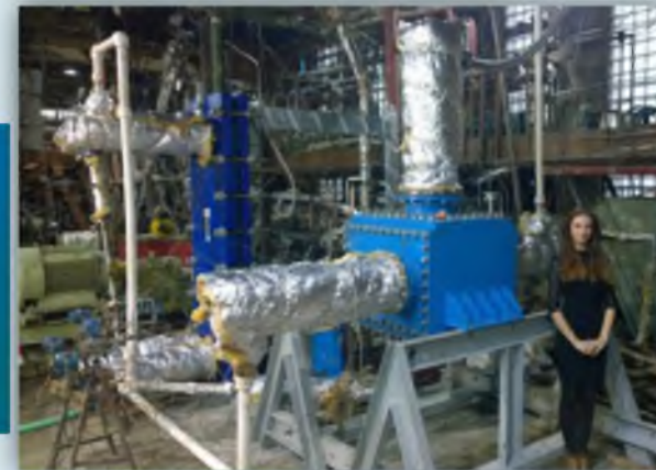
Recirculation cooling plant RCP-6.3 EMK.0155.000.00.000 for the third unit of the Rostov Nuclear Power Plant (emergency mode emulation)
