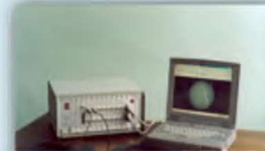
Acoustic emission diagnostics system SDAE-16
