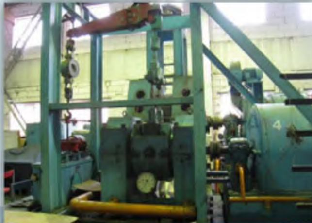
Test rig for journal bearing with diameters up to 450 mm investigation
