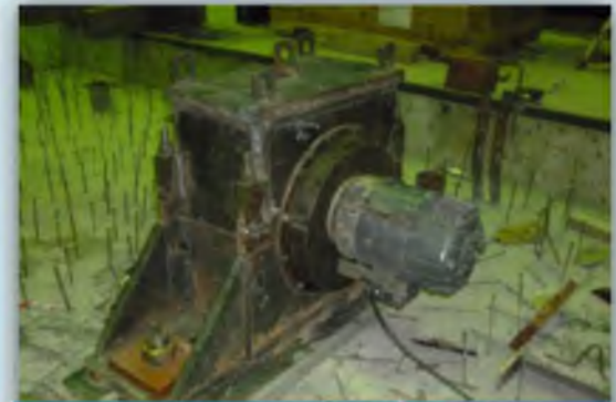
Vibrating unit installed on examined foundation
