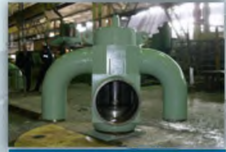
FSD valves (inlet and outlet)
