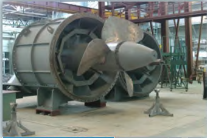
Variable-speed hydroelectric unit for Mitu HPP (Colombia)
