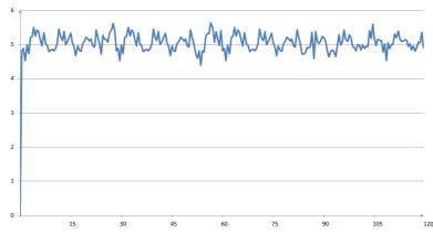
Graph 2 Start-up graph: Flow rate 5 (ml/h)against time (min) plotted from data gathered during the first 2 h of the test period
