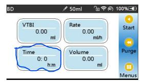
Under this mode, it allows to set three parameters: Rate, VTBI (Volume to be infused) and Time, set any two of the three parameters, and the system will automatically calculate the third parameter, if the VTBI is 0, then the equipment works at the set rate till stop with alarm.
