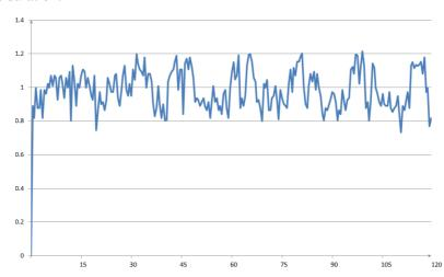
Graph 1 Start-up graph: Flow rate 1 (ml/h) against time (min) plotted from data gathered during the first 2 h of the test period
