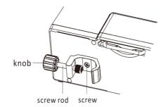
(2) Lock the Pole Clamp on the infusion stand, adjust the position of the syringe pump, tighten the pole clamp to fix the syringe pump on the infusion stand (shown in drawing below). Hold the syringe pump when tightening the fixing clamp; loose it after tightening to avoid falling.
