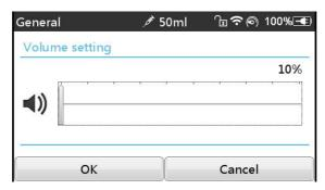
Click  $\lceil$  Sound  $\rfloor$  to enter into the sound parameters setting interface, the volume has 10 levels. The lowest volume is  $\geq$ 50dB, and the highest volume is  $\leq$ 80 dB. Move the long box to the preset value, after confirming, click  $\lceil$  OK  $\rceil$  .
