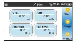
Ramp up/down mode means to automatically increase the flow rate till reaching stable flow rate within the set rising time of the equipment through setting the rising time and falling time, after holding for a period, it automatically drops the flow rate within the set dropping time. The rising or dropping stage is implemented in 9 stages.
