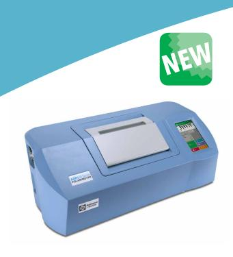
Available as single, dual and multiple wavelength derivatives covering the visible spectrum, the ADP600 Series also features measurement in the highly sensitive ultra-violet region. This capability makes the instrument particularly suited for use by scientists wishing to measure chiral compounds and other optically active substances in the chemical, pharmaceutical and food sectors as well as for use in academic research.
