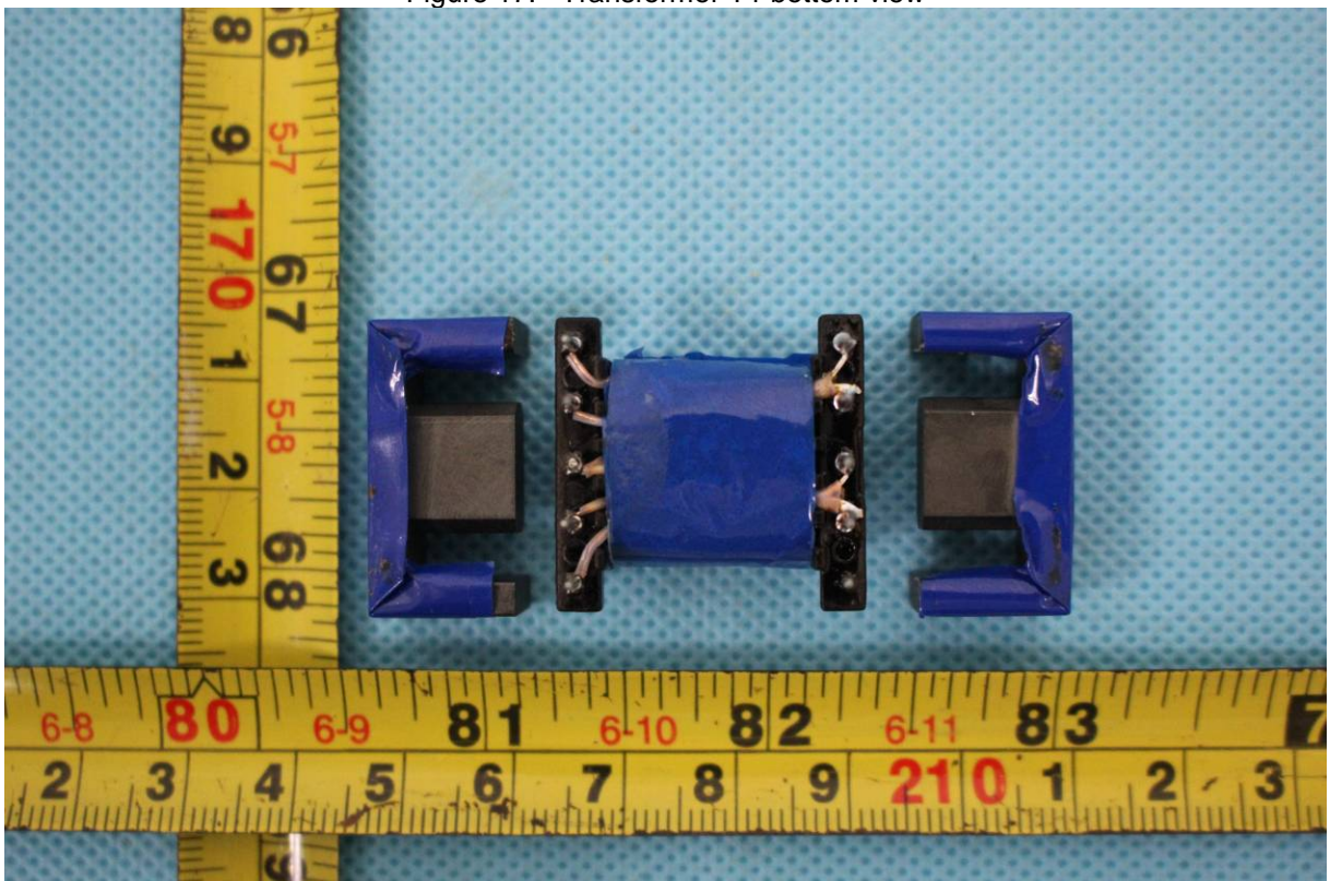
Figure 18. Transformer T1 bottom view (two layers insulation tape wrapped over transformer core)
