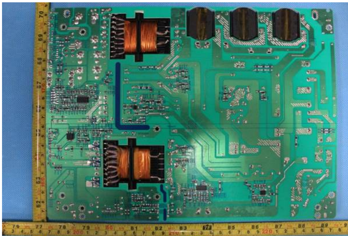
Figure 9. Power board PCB trace side view (with mylar sheet removed)
