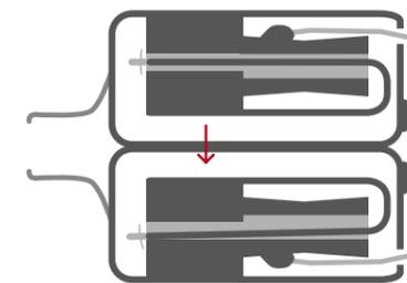
Bendt armature due to high impact
