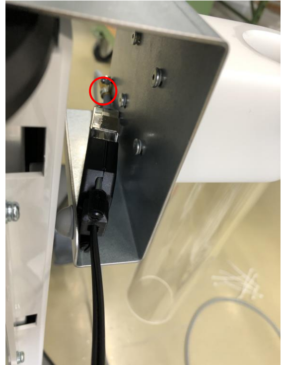
Figure 6: fiber optic converter to StormLink cable fixed with a cable clamp
