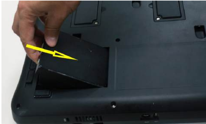
Figure 3-39. Place the battery in the battery box
