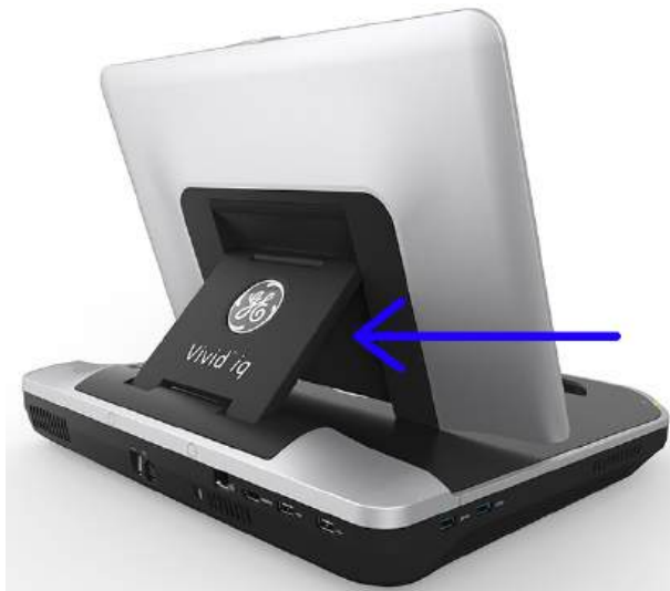
Figure 3-8. The pinch point
