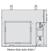
\* The heavy-duty auto drain and piping materials (nipple, elbow) are shipped together with the main body of the air dryer. Customers are required to mount the parts to the air dryer.
