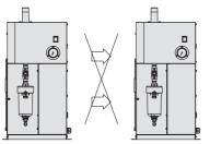
Confirm that the exhaust air does not flow into the neighbouring equipment.
