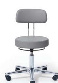
WORK CHAIR 40 - 52 cm. Item code 3018105 5-star base polished, small backrest height adjustable, sitting cushion Ø 36 cm, cover in compact „Stone“ C214, 360° manual ring release, safety castors.
